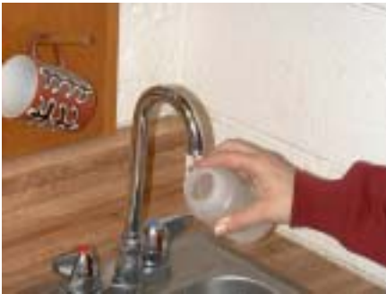
Sampling at the tap for bacteria in well water.
