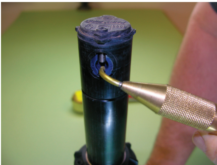
Figure 20: Insert the pitot tube in the water stream.
