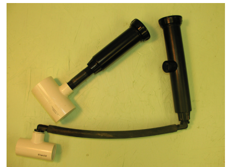
Figure 7: Swing pipe and nipple extension.
