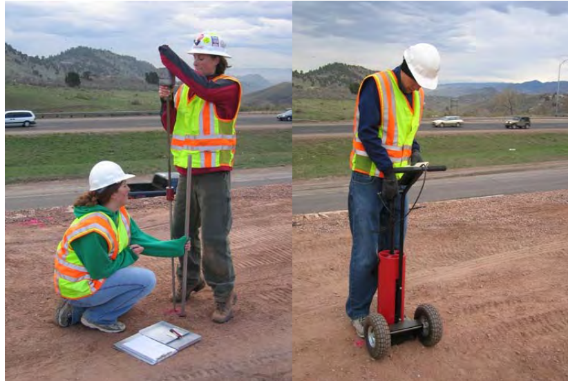
Figure 3-3. DCP and Clegg Impact Hammer Operation
