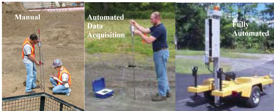
Figure 2-2. Manual, Automated Data Acquisition, and Fully Automated DCPs (right two photographs from Vertek, 2006)
