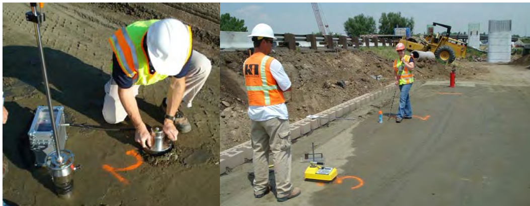
Figure 3-3. DCP and Clegg Impact Hammer Operation
