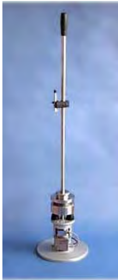
Figure 2-7. Dynatest 3031 LWD (left) and Zorn ZFG 2000 LWD (right)
