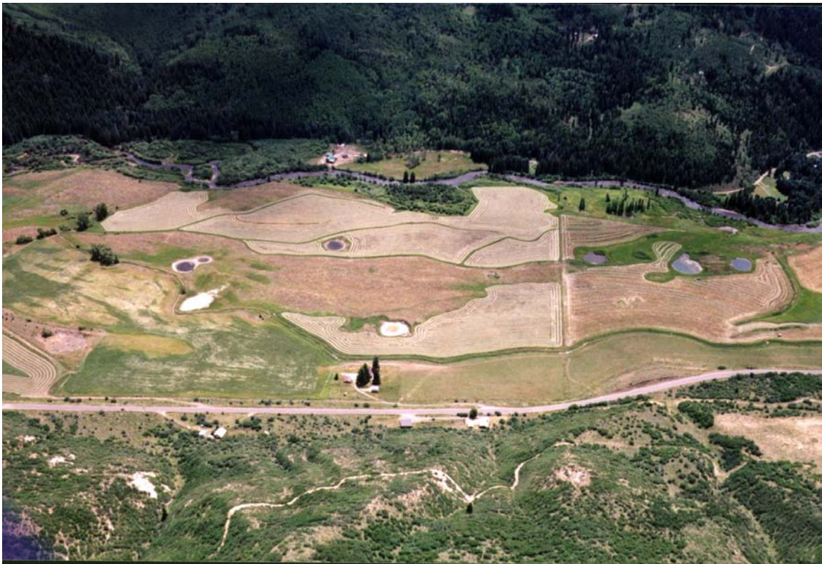
Figure 2. Several sinkholes give Pothole Ranch its name where the Eagle Valley Evaporite is near surface along the North Fork White River valley about 4 miles east of Buford in Rio Blanco County.
