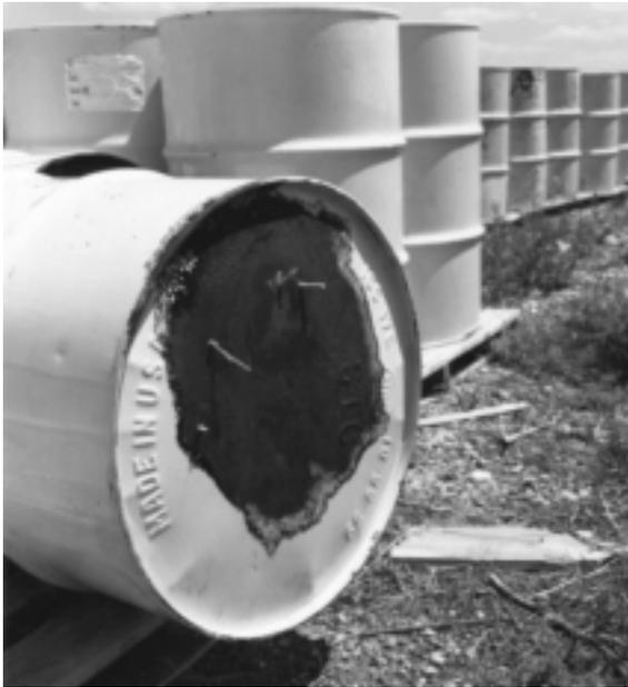
Barrels corroded and leaked plutonium-contaminated oil onto soil. Weeds grew through the badly corroded bottoms of these barrels.
