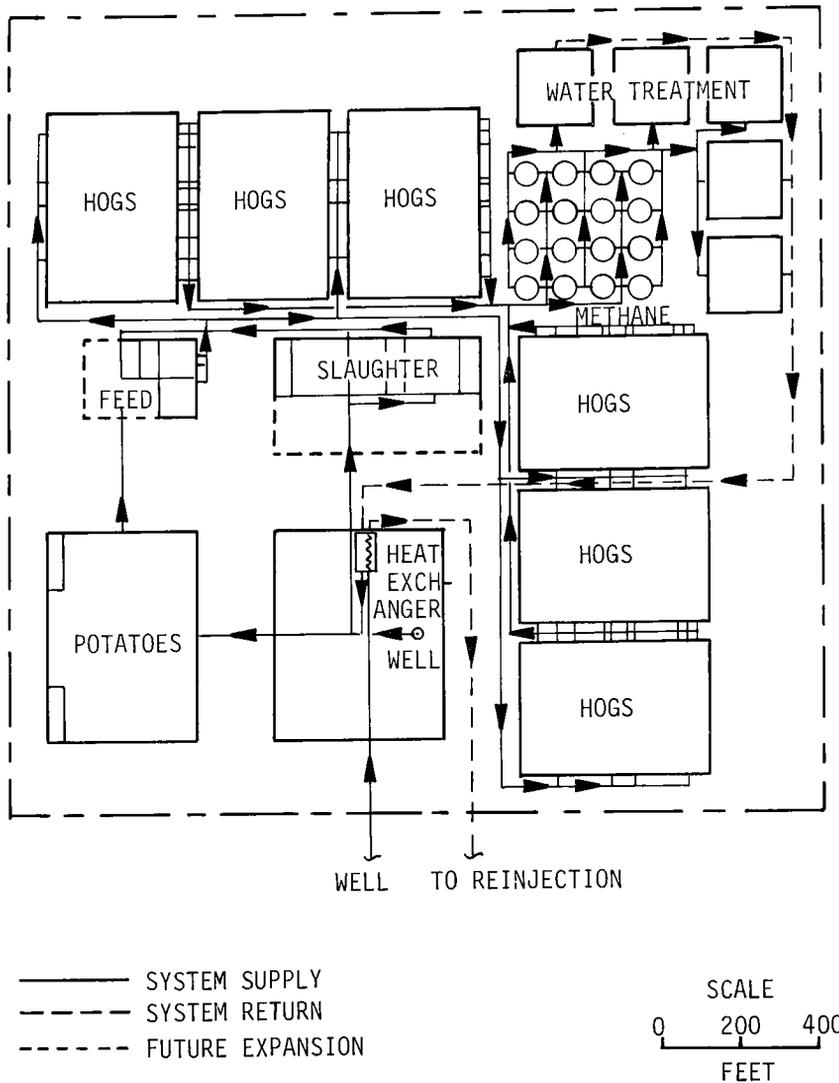
Figure 9. Schematic Diagram of Hot Water Mains for Integrated Livestock and Feed Production Facility (from Energetics and Marketing and Management Association, Ltd., 1979).
