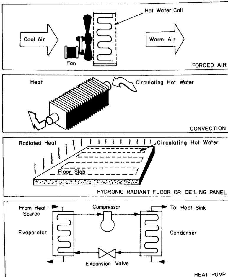
Figure 4. Types of Heating Systems Suitable for Geothermal Applications (from Lienau, 1979).
