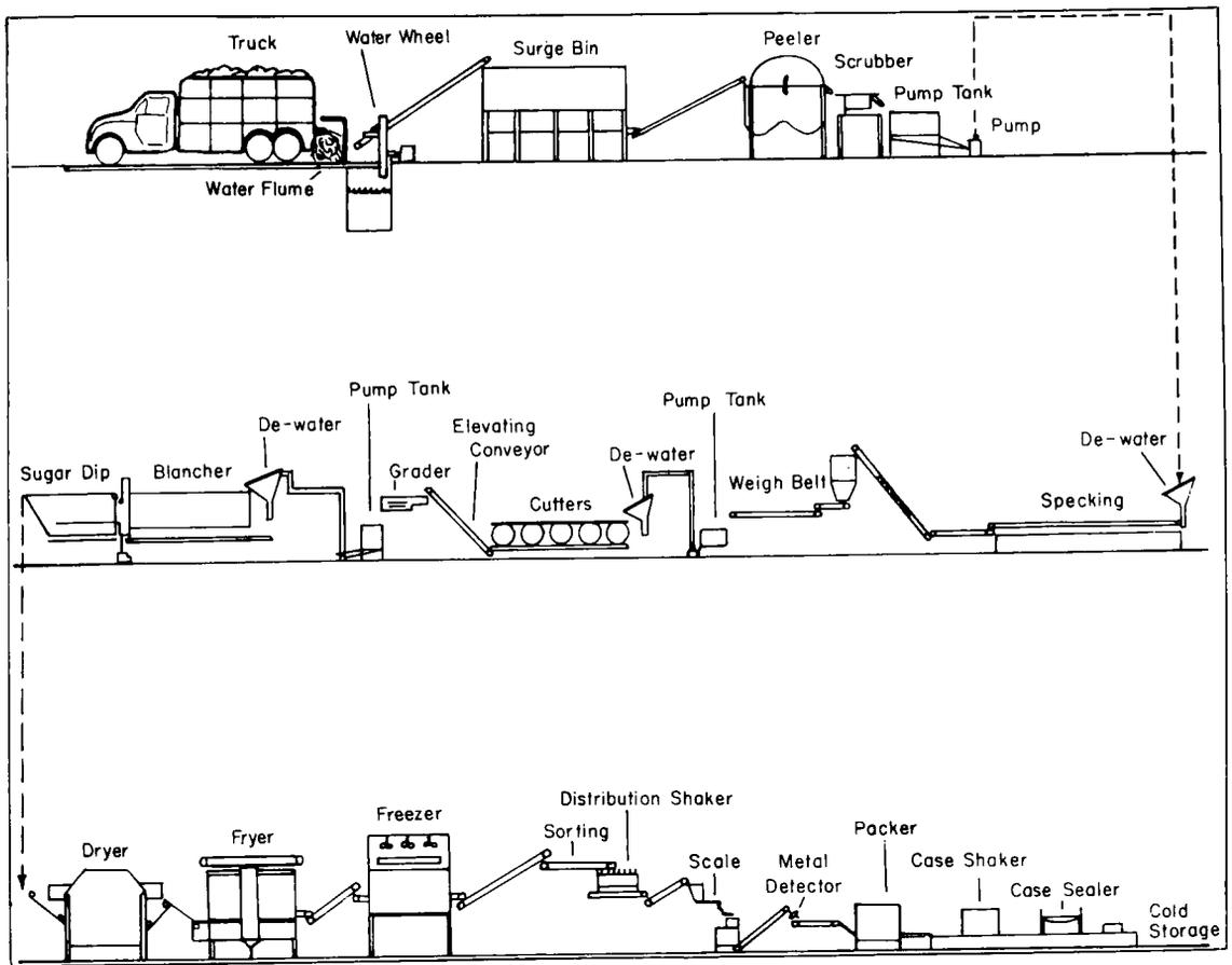
Figure 16. Potato Processing Schematic (from Lienau, 1979).
