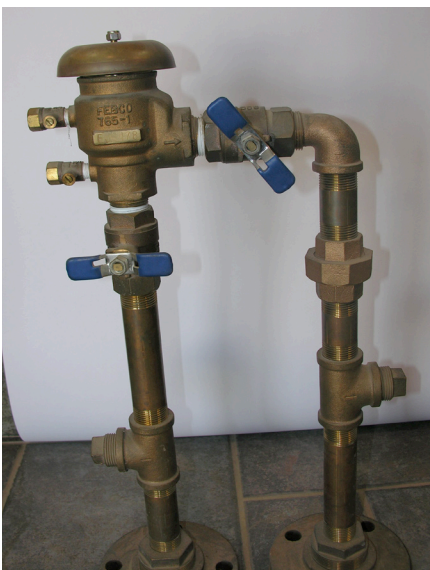
Figure 3: Left Photo – Pressure vacuum backflow device (PVB) Right Photo – Reduced Pressure backflow device (RP). Blue handles designate isolation ball valves. Note blowout fittings (tees with threaded plugs) on either side of the device.
