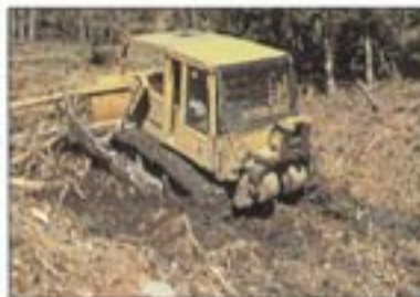
Stay clear of wet areas during scarification. Results like this create compaction and water quality problems.
