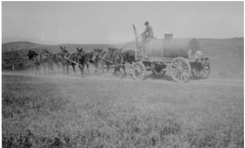
Tank hauling fuel: capacity 17 barrels; total load 3.5 tons. Courtesy of the Bancroft Library, University of California, Berkeley 19xx.129—ALB, container 4, Image 35.
