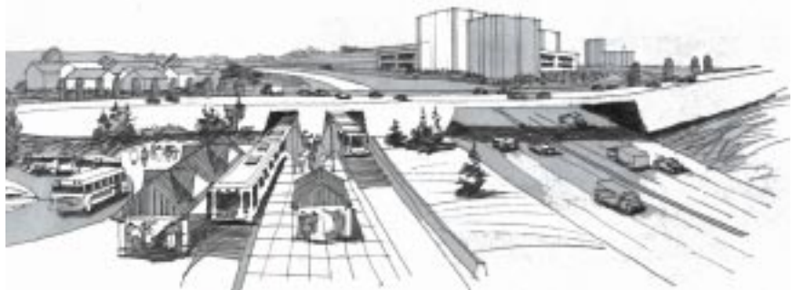
Figure 2-15. Bellevue Station from the air, looking north. Shown is the bus plaza west of the platform and the Union Avenue bridge north of the station. Transit patrons will be able to access the station via stairs and an elevator at the bridge.
