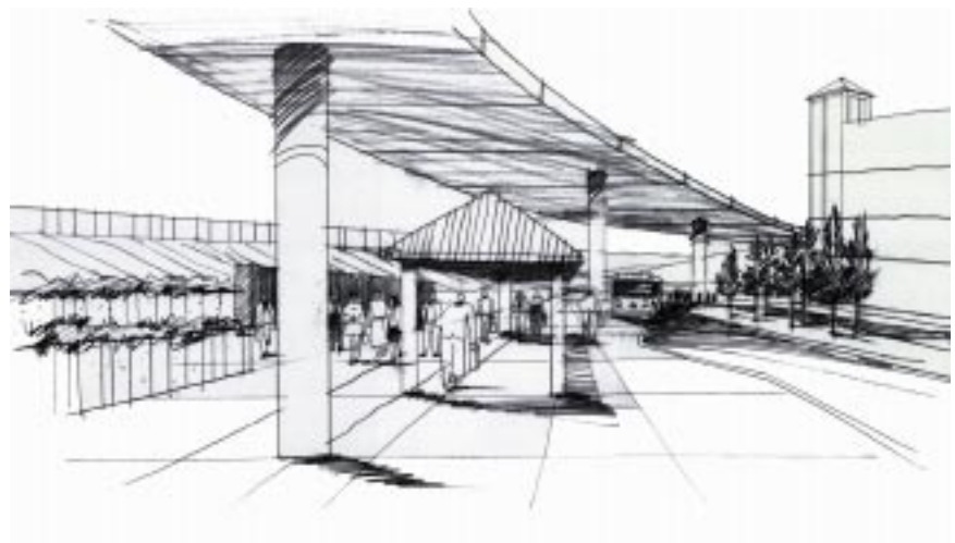
Figure 2-29. The Nine Mile Station will be located in the middle of a loop ramp from I-225 to Parker Road (shown above bus plaza). The light rail platform, located in the median of the highway will be accessible via underpass.
