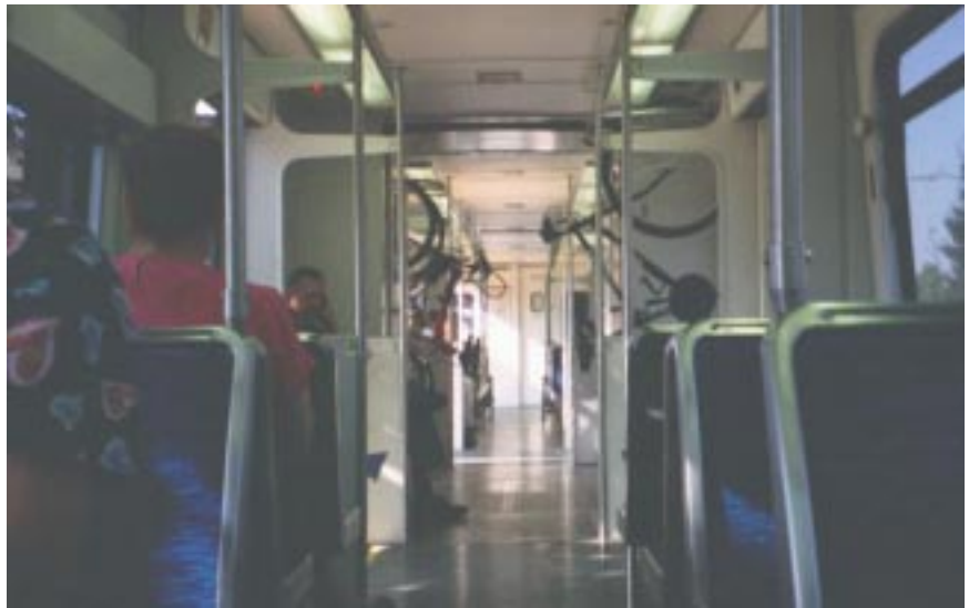
Figure 4-1. Interior of a Santa Clara VTA light rail train. The bike racks are located near the articulation in the train car, with overhead hooks to which bikes are hung.
