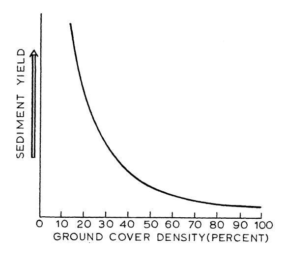
Fig. 1. Generalized schematic of sediment yield as a function of ground cover density.
