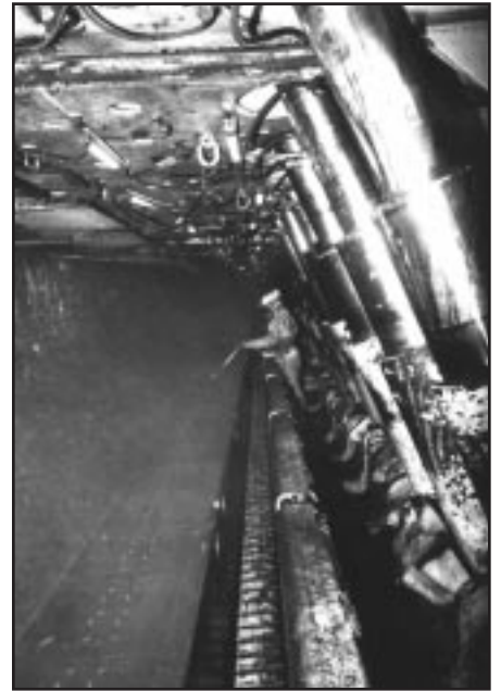
Longwall machine at the West Elk Mine. Photo courtesy of Wendell Koontz, Mountain Coal Co.
