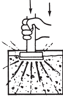
FIGURE 2.5-6 TRANSMISSION OF COMPACTION FORCE
