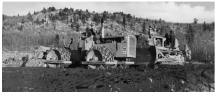
FIGURE 2.5-10—SELF-PROPELLED ROLLER.—Used in open areas.
