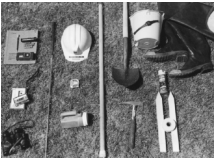
figure 4.2-1 inspection equipment—Notebook, pencil, hand-level, camera, tape recorder and tape, binoculars, probe, hard hat, pocket tape, flashlight, bonker, shovel, rock hammer, bucket and stopwatch, bug spray, flagging tape and stakes, waterproof boots.
