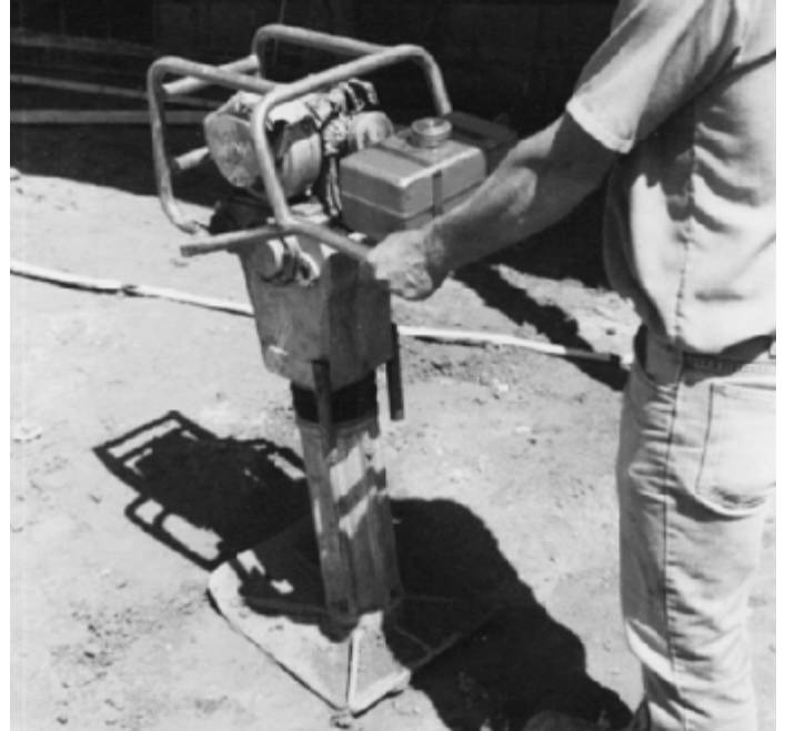
FIGURE 2.5-8—WACKER.—Is used in areas larger equipment cannot reach.
