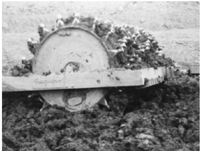
FIGURE 2.5-9—SHEEPSFOOT ROLLER.—Used in open areas.
