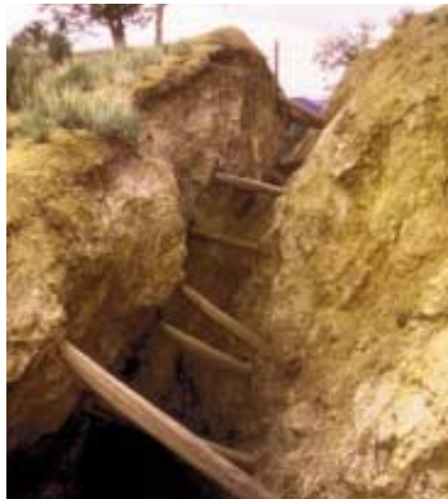
STOPE SHOWING STULLS SUPPORTING HANGING WALL
