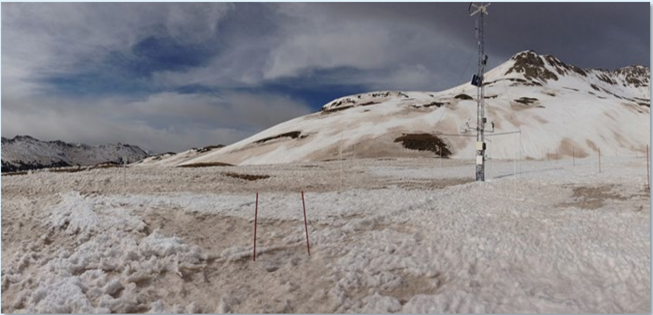
View of the Senator Beck Study Plot at the Center for Snow and Avalanche Studies (CSAS), San Juan Mountains, Colorado, on May 5, 2013. The dark patches where that season's extreme dust accumulation has emerged at the surface sit lower than the adjacent cleaner snow, indicating the enhanced melt rate due to the dust. (Photo: CSAS Colorado Dust-on-Snow program.)
