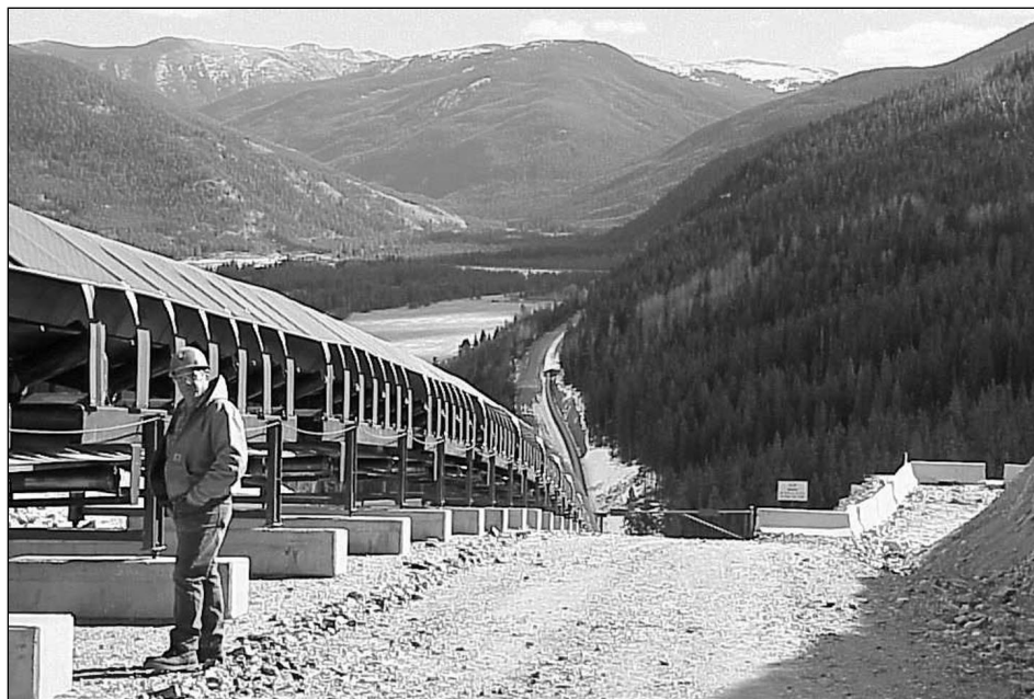
Portion of the surface conveyor belt between the Henderson Mine and the mill—PHOTO COURTESY OF HENDERSON MINE
