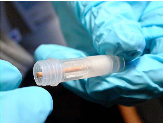
FIGURE 3. Insert swab or stick into tube with sample at bottom of tube.
