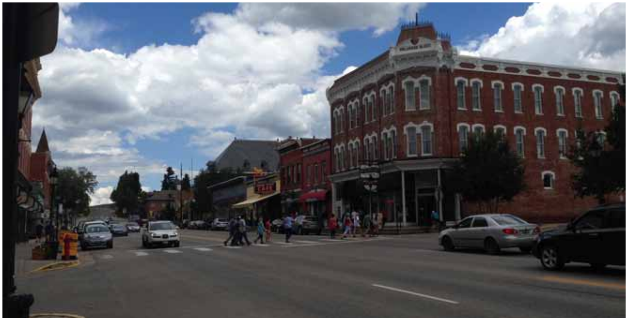
Marked crosswalks reinforce pedestrian right-of-way at intersections, enhance safety and visibility, and can be located at mid-block crossings as well. Leadville.
