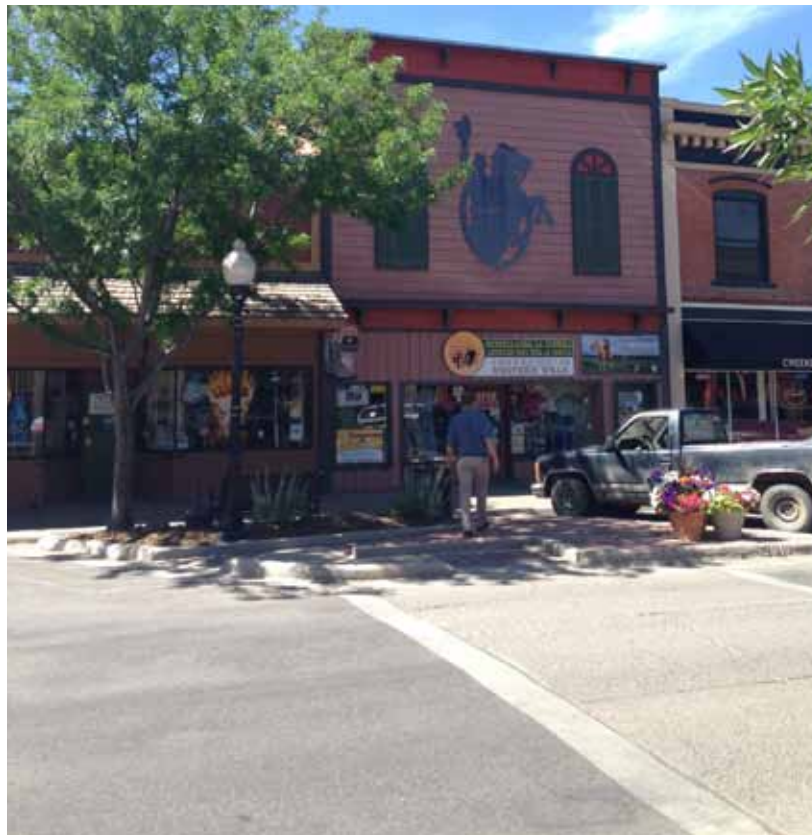
In the appropriate locations, midblock crossings provide safe, visible locations for pedestrians to cross the street away from intersections. Rifle.
