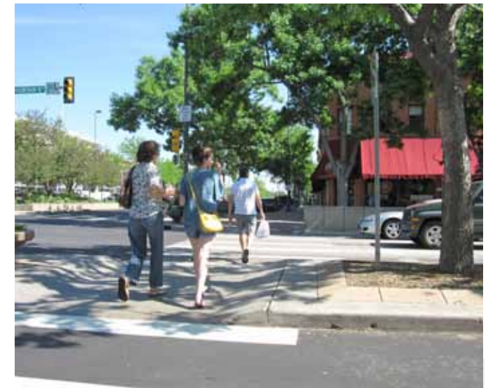
Refuge islands provide a protected area for pedestrians within the travelway. Fort Collins.
