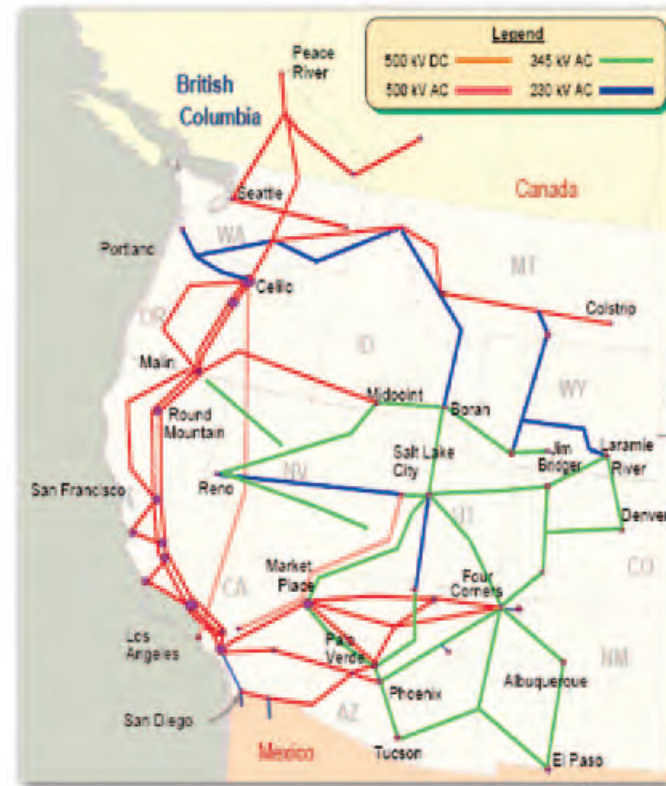
Figure 2-3: Primary Components of the WECC Transmission Grid
