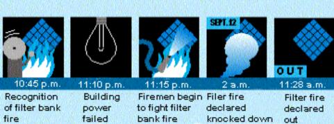
Although plutonium burns slowly, much like charcoal, the heat generated caused material in a glovebox, and the plastic walls of the box, to catch fire. The fire destroyed many of the paper filters in the filter bank that were designed to prevent plutonium from escaping into the atmosphere through the building's stack. The destruction of the filters allowed plutonium dust and smoke to go directly into the environment.
