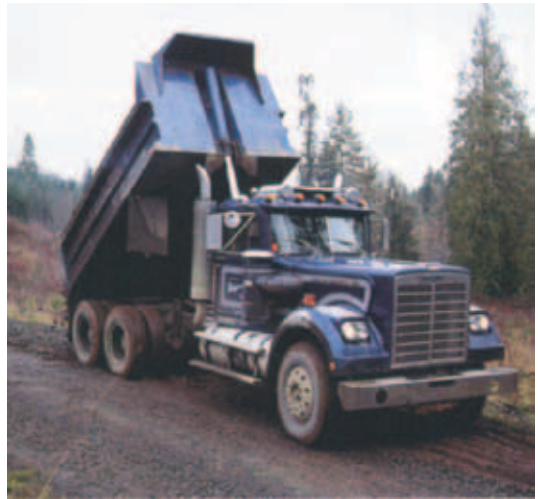
Figure 6-1. Dump truck placing aggregate on road.
