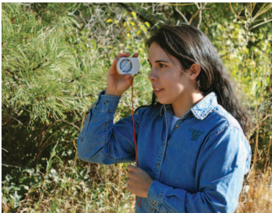
Figure 1-19. Measuring road grade with a clinometer. Photo: Lisa Mason
