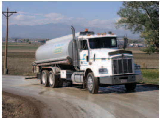
Figure 5-52. A dust-suppressant spray truck applying magnesium chloride.
