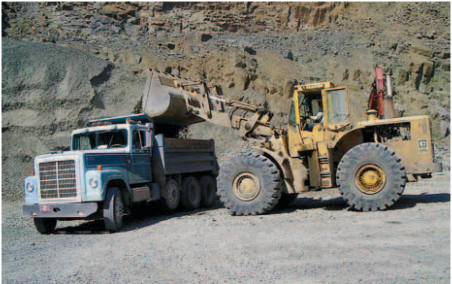
Figure 1-14. Front-end loader and dump truck at rock quarry.
