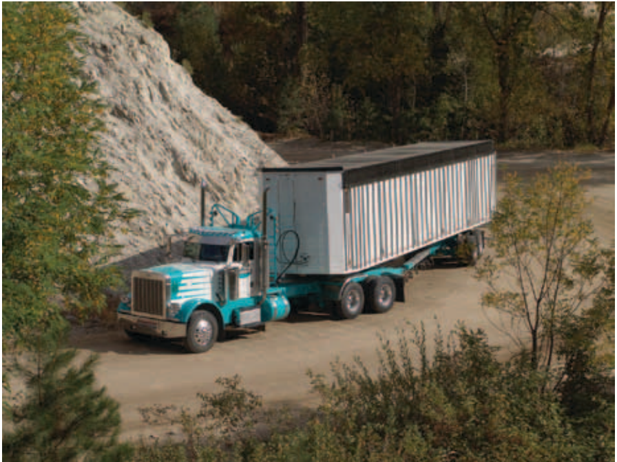
Figure 2-15. Stinger-steered chip trailer negotiating curve. Photo: Western Trailers
