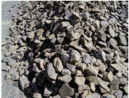
Figure 3-9. Coarse, clean rock suitable for ditch armoring.
