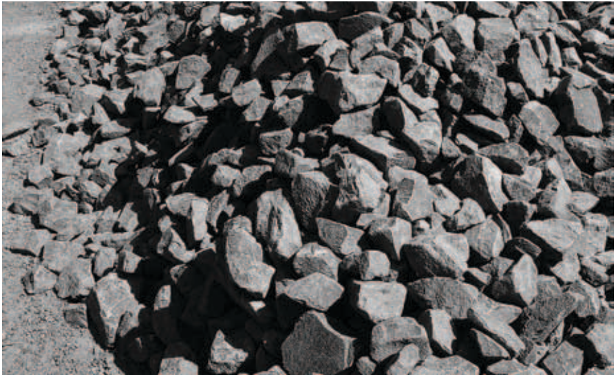
Figure 1-12. Example of angular, clean and durable rock.
