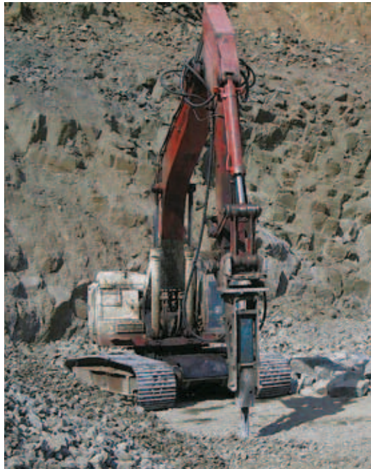
Figure 1-13. Excavator with hydraulic rock breaker.
