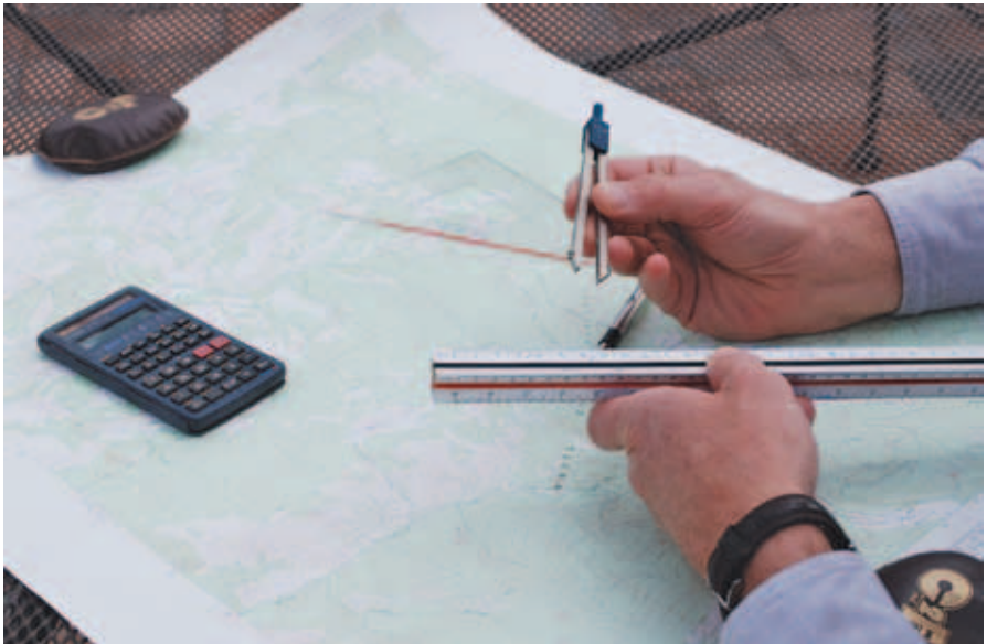
Figure 2-7. Mapping equipment needed for direct layout/road location. Photo: Lisa Mason
