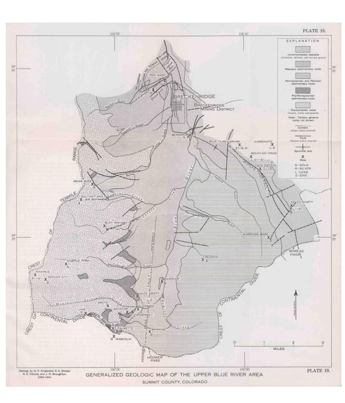
section of the two belts, one longitudinal and the other transverse, of relatively intense pre-Cambrian deformation. The Hoosier Pass structure, which includes a major longitudinal fold and an inferred fault, crosses the eastern part of the area; it doubtless had some influence on the general distribution of ore, yet it cannot be regarded as the dominant controlling structure.
