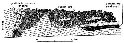
FIGURE 8.—Sketch showing replacement of rubble, sand, and bedrock in ore channel at Gilman. Mineralogic zoning is parallel to contact of ore body and independent of textural types.
