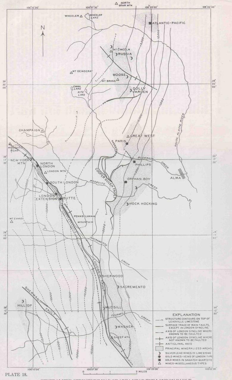
GENERALIZED STRUCTURE MAP OF AREA NEAR THE LONDON FAULT, SHOWING RELATION OF ORE DEPOSITS TO MAJOR STRUCTURE.
