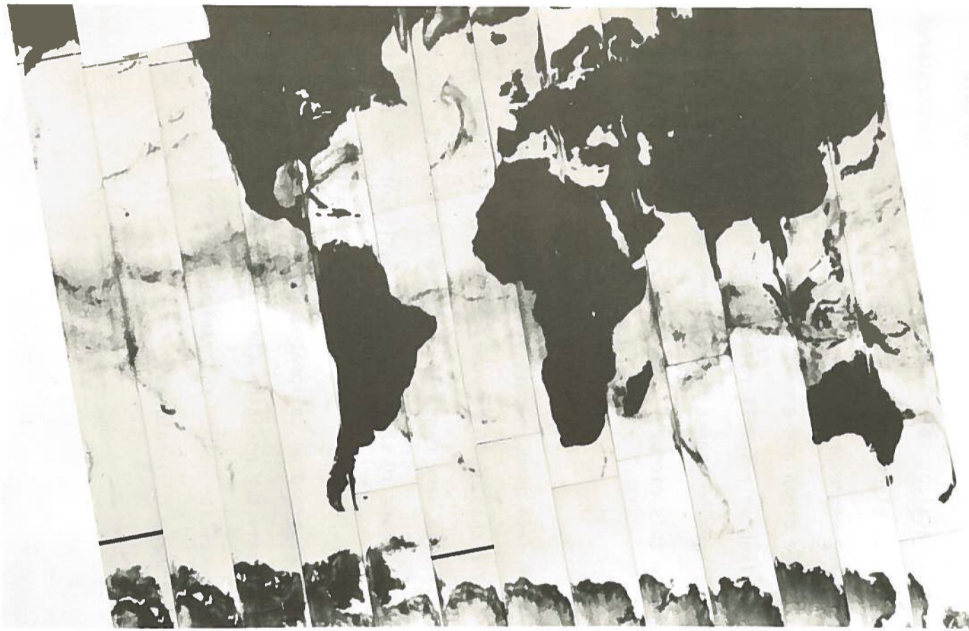
Figure 9. Photographically processed Nimbus 5 ESMR data from 11 January 1973, orbits 413-425. Brightness temperatures less than 190 K are white, those greater than 250 K are black, and those in between are represented by a linear gray scale. Rain, which appears dark over the ocean is evident in the tropics and in several weather fronts. (From The Nimbus 5 Data Catalog , Vol. 1)
