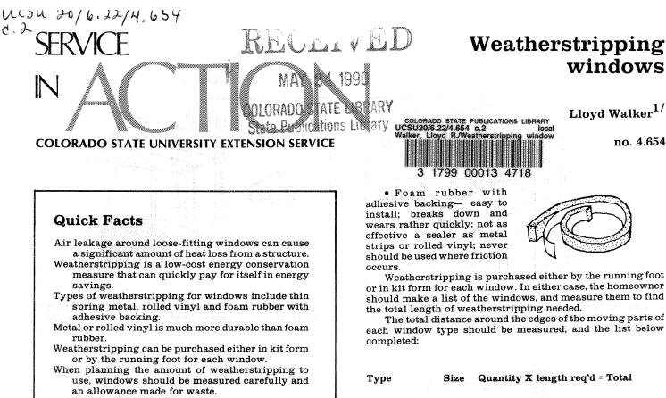
Air leakage around loose-fitting windows can cause a significant amount of heat loss from a structure. Weatherstripping can seal these air leaks. It requires a minimum of simple tools and no specialized skills. Weatherstripping is a low-cost energy conservation measure that can quickly pay for itself in energy savings.
