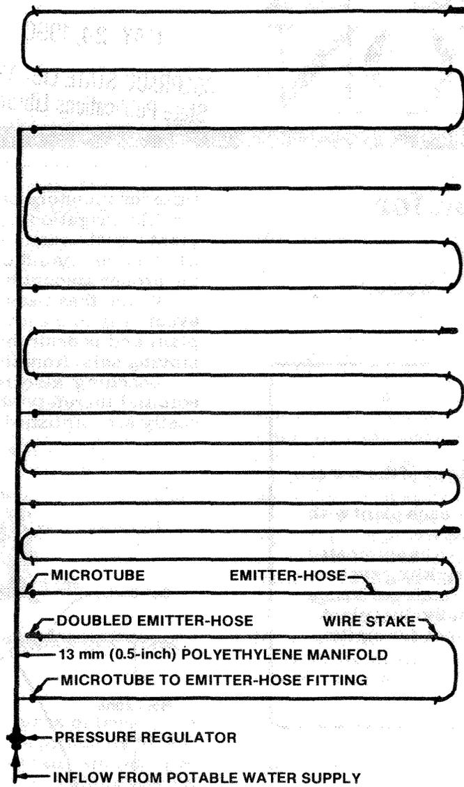
**Figure 4: Layout of a drip irrigation system compatible with the garden depicted in Figure 3.**
