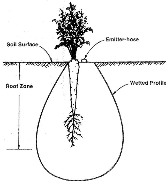
Figure 1: Idealized wetted profile below a "trickler" or "emitter."
