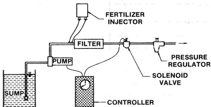
Figure 2: Typical trickle system "head."
