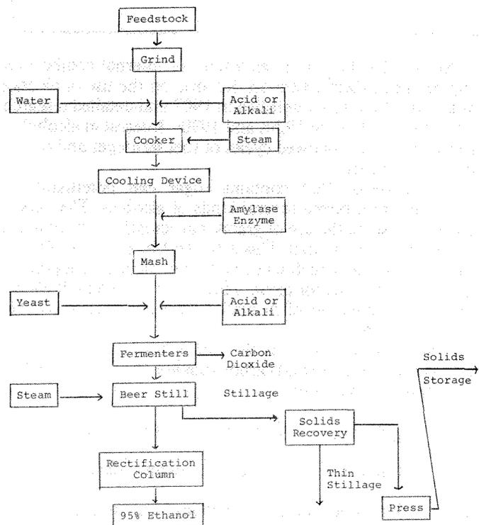
Figure 1. Alcohol production flow chart (190 proof ethanol).
