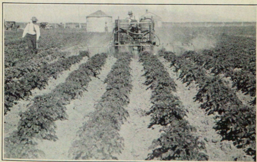
Figure 15—A front view of the sprayer shown in figure 14, showing the six-row boom.
