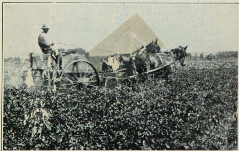
Figure 16—A four-row power sprayer in the San Luis Valley doing a good job of spraying. The foliage in this field was very heavy, but with high pressures and sufficient delivery capacity the field was thoroughly sprayed and psyllids were controlled.
