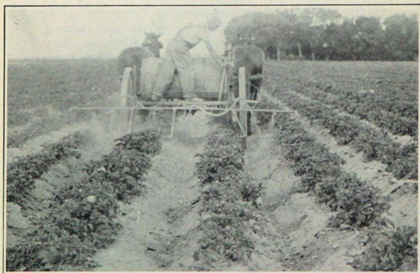
Figure 10—A low-pressure traction sprayer in operation. This type of machine is being replaced by the power sprayer in controlling potato insects.
