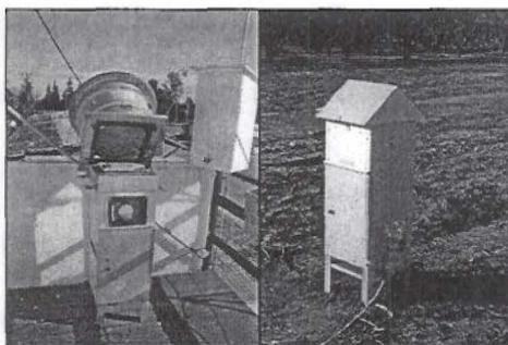
**Figure 2. Hi-Vol instruments with a PM<sub>10</sub> inlet (left side) and without a PM<sub>10</sub> inlet (right side).**
