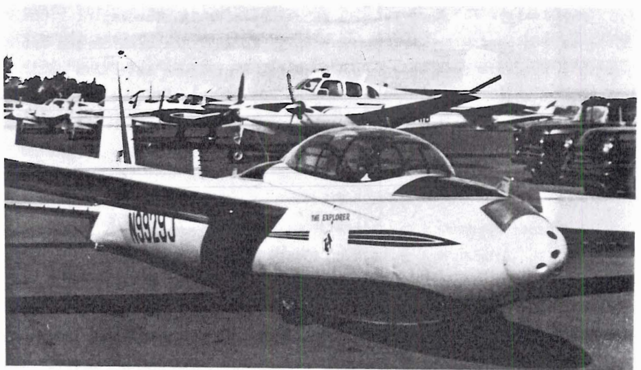
Figure 1. The Explorer sailplane. Location of the temperature ensor denoted by 1. The ozone sensor intake is located on opposite ide of fuselage.
