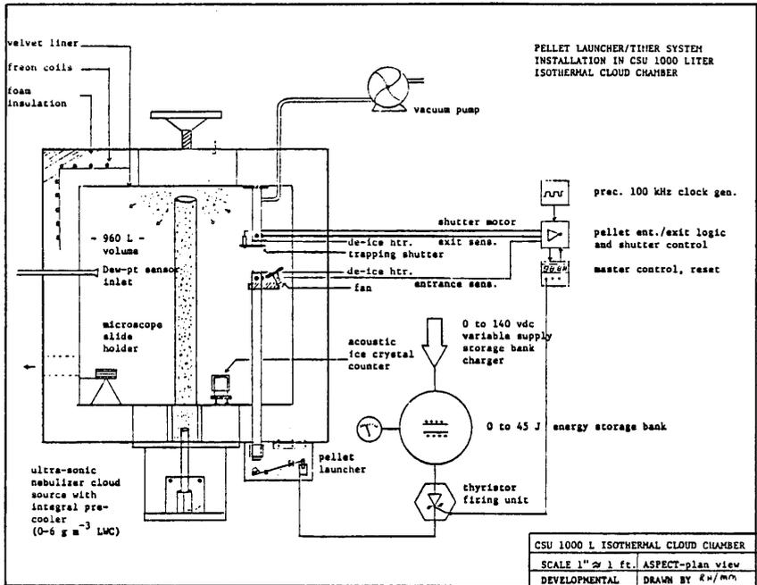
Figure 1. Schematic of 960 liter Isothermal Cloud Chamber and apparatus used in the dry ice pellet experiments (not to scale).
