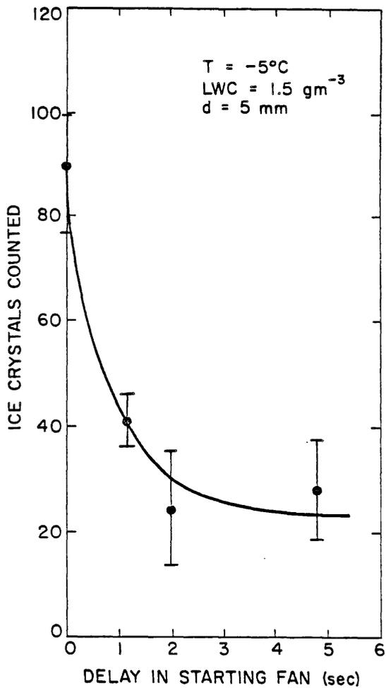
Figure 6. Test for aggregation of ice embryos in the dry ice pellet plume.
