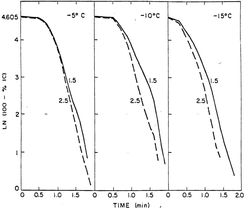
Figure 19. Composite kinetics plots for 5 mm dry ice pellets at  $1.5$  and  $2.5 \text{ g m}^{-3}$  cloud liquid water contents. Pellet velocities are approximately  $12.3 \text{ m s}^{-1}$ .
