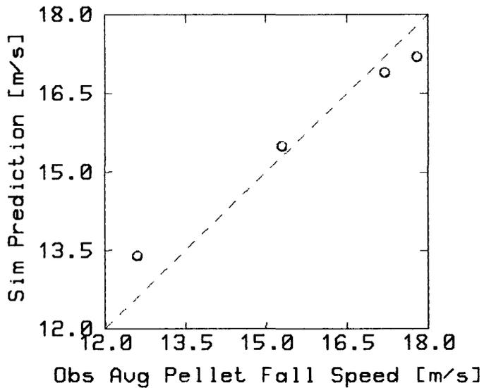
Figure 10. Observed dry ice pellet fall speeds from clear air drop experiments versus simulation prediction.
