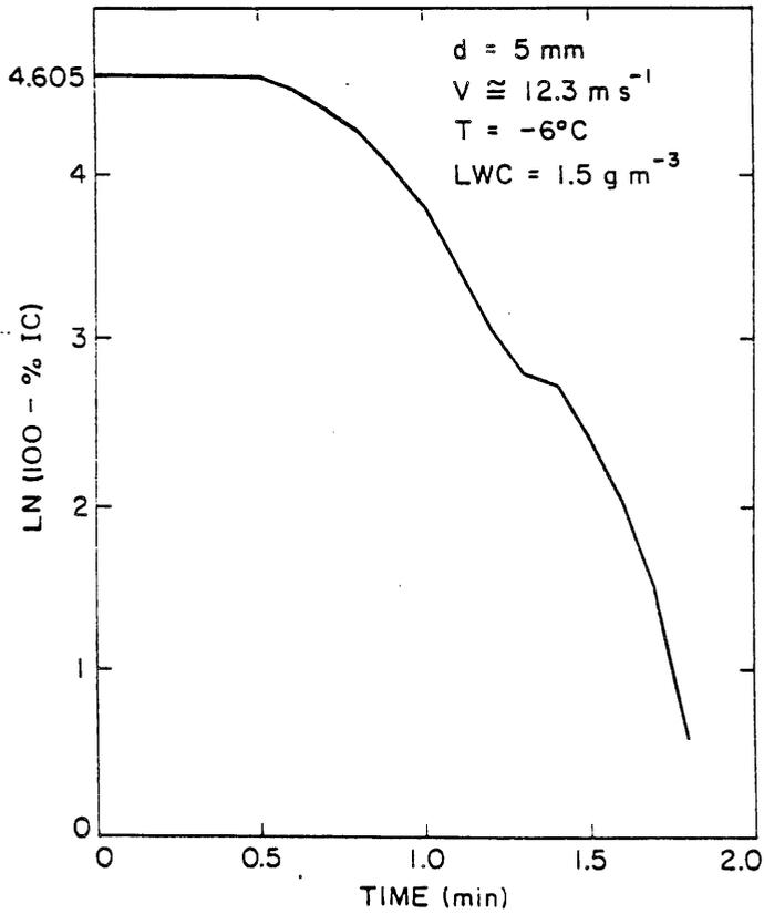
Figure 9. Composite kinetics plot formed from the plots in figure 8.
