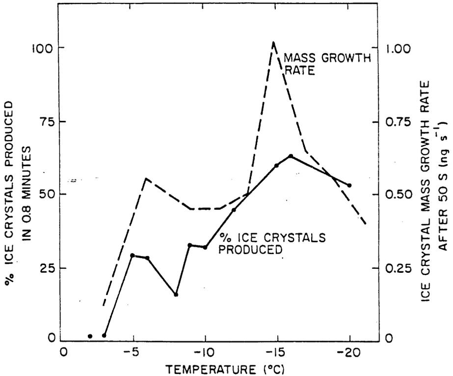
Figure 16. Percentage of the total number of ice crystals counted that were observed in 0.8 minutes for 5 mm dry ice pellets at a cloud liquid water content of  $1.5 \text{ g m}^{-3}$  (solid line). The pellets velocity was  $12.3 \text{ m s}^{-1}$ . The mass growth rate for ice crystals after Ryan *et. al.* (1976) is plotted as the dashed line.
