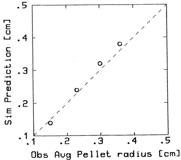
Figure 11. Observed dry ice pellet radius from clear air drop experiments versus simulation prediction.
