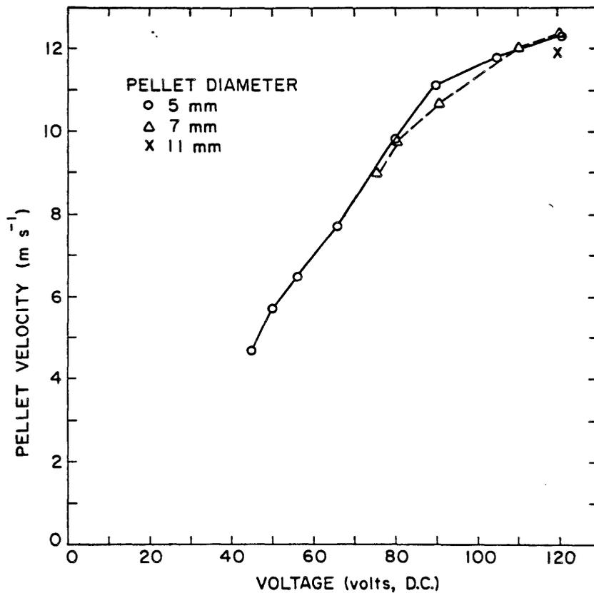
Figure 4. Pellet speed calibration curves as a function of solenoid voltage for three different pellet sizes.
