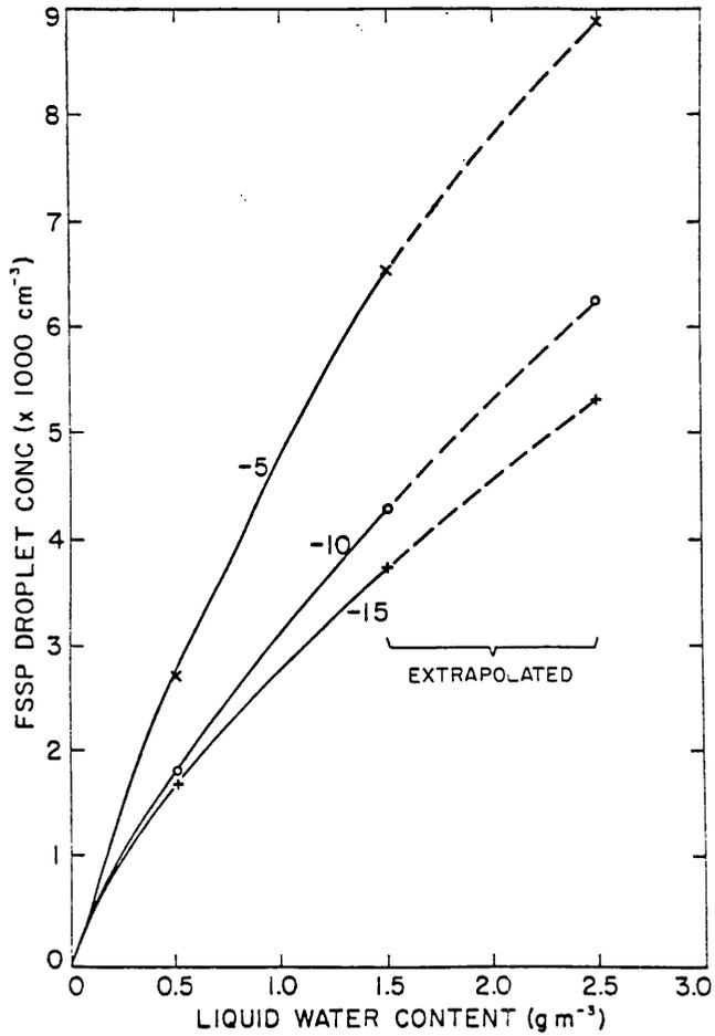
Figure 18. Extrapolation of cloud droplet concentrations for -5, -10, and -15 °C at a cloud liquid water content of 2.5 g m<sup>-3</sup>. The data points at 0.5 and 1.5 g m<sup>-3</sup> were taken from figure 3. The curves shown are hand-fitted.
