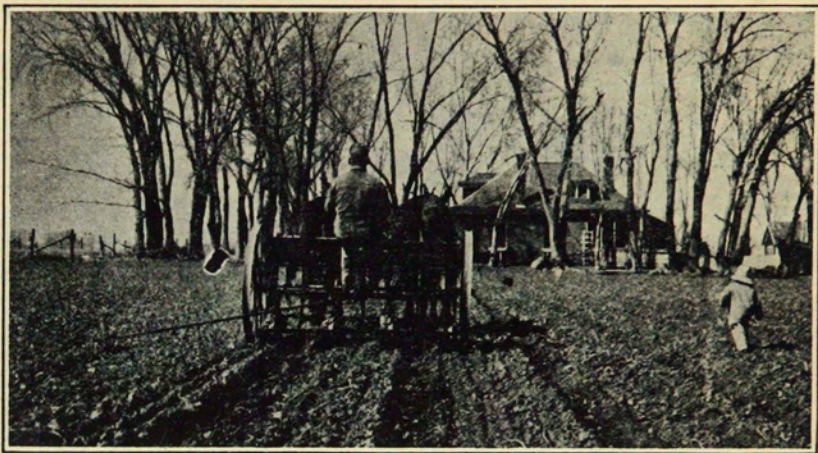
Using furrow openers on a beet drill permits early cultivation or irrigation.
