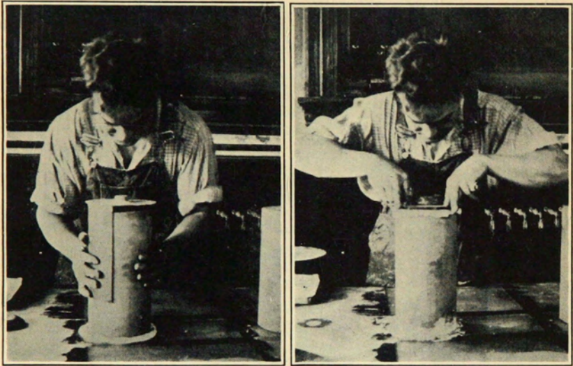
Fig. 6.—Left. Setting cylinder vertical on horizontal glass plate while applying lower cap. Right. Leveling upper glass plate while applying cap to the upper end.
