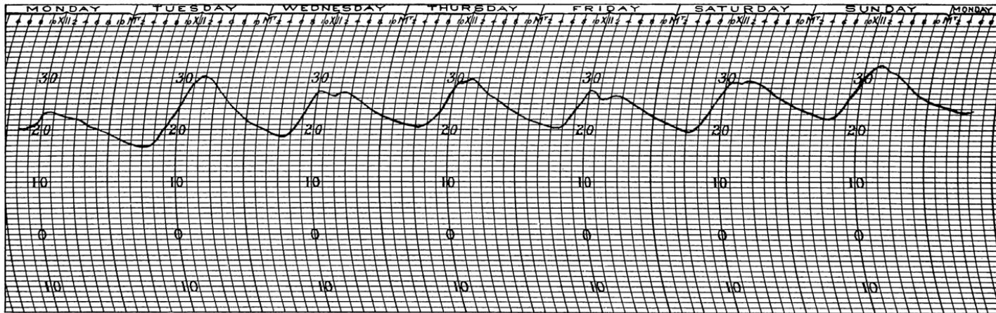
Fig. 7. Soil thermograph record for the week July 21 to 28, 1930, in degrees Centigrade.
