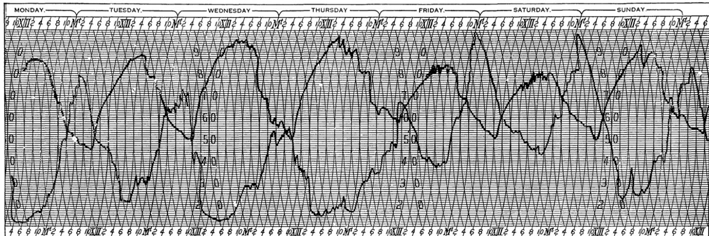
Fig. 5. Hygrothermograph record for the week June 25 to July 2, 1930, in degrees Fahrenheit.
