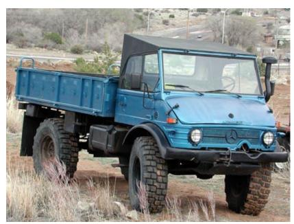
This German-made "Unimog" purchased by Gila WoodNet is an example of the smaller, more manueverable, and low-impact machinery being employed in small-diameter restoration logging.
