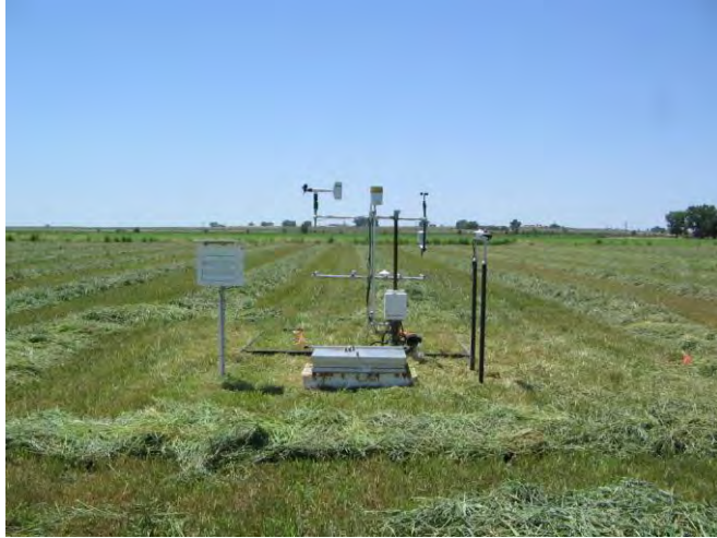
Figure 5. View of the lysimeter and meteorological instrumentation in late June 2007. Photo taken by Michael Bartolo.
