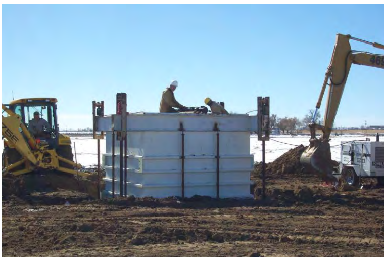
Figure 1. The inner tank being pushed into the ground to acquire the soil monolith. Photo taken by Dale Straw of DWR.
