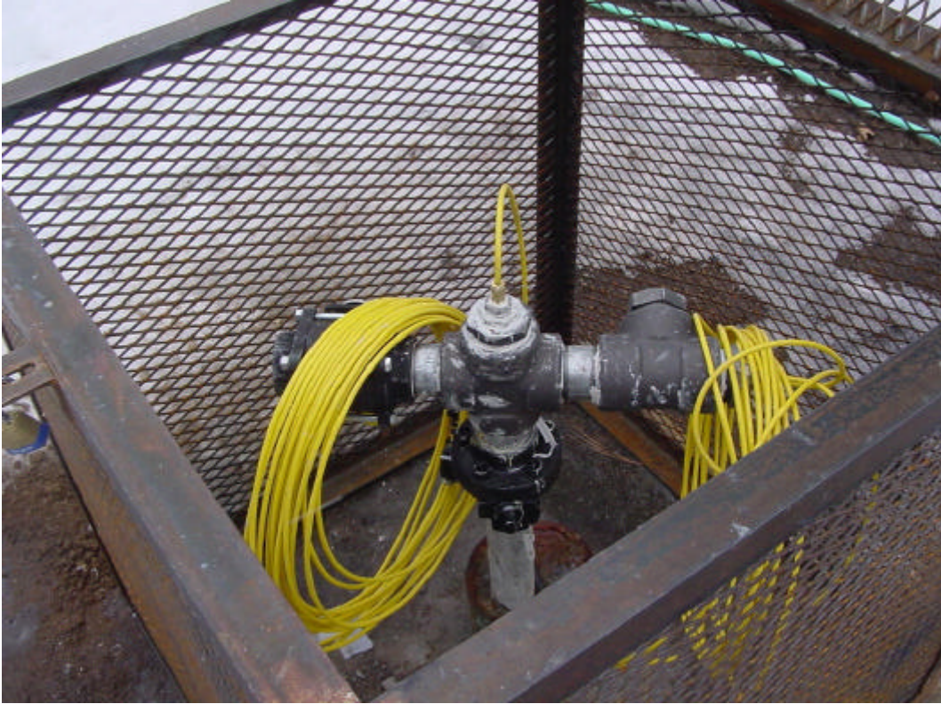
Photo 3. Beaver Creek Ranch MW 35-6-17-2 wellhead assembly.
