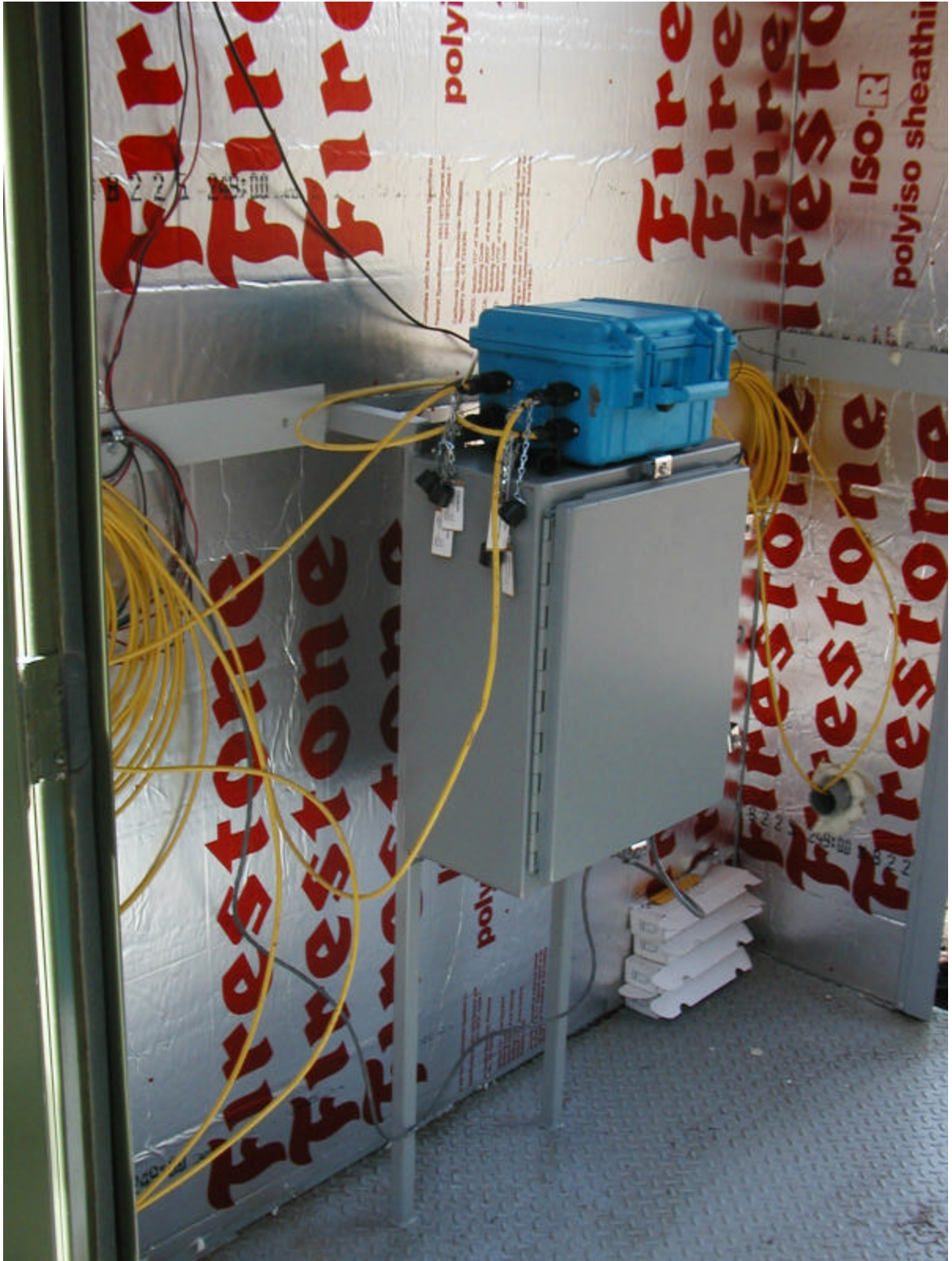
Photo 7. Hermit logger and telemetry at South Fork of Texas Creek (final).
