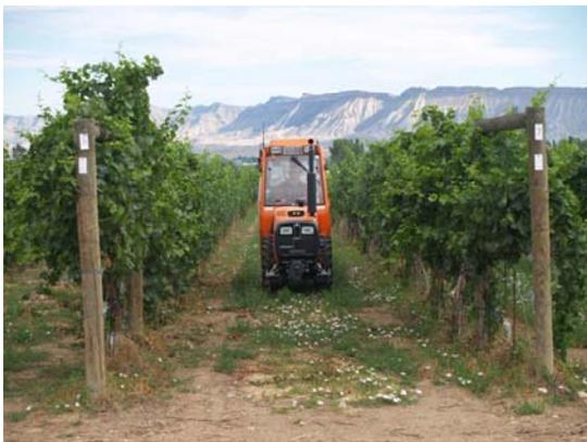
Test of narrow (3 ft) vineyard tractor and sprayer for use in ultra-high density vineyards. WCRC-Orchard Mesa, Grand Junction,
