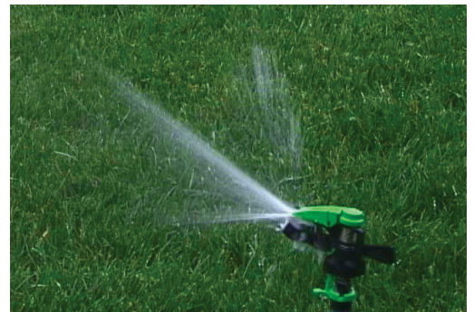
Figure 3. Impact or impulse heads rotate as the water stream coming from the nozzle hits a spring-loaded arm. Impact heads tend to experience fewer problems under marginal (dirty) water quality.
