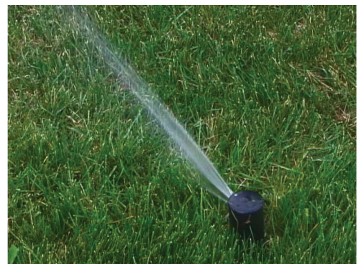
Figure 4. Gear-drive heads use the flowing water to turn a series of gears that rotate the head. Compared to the impact heads, gear-drive heads are quiet to operate.
