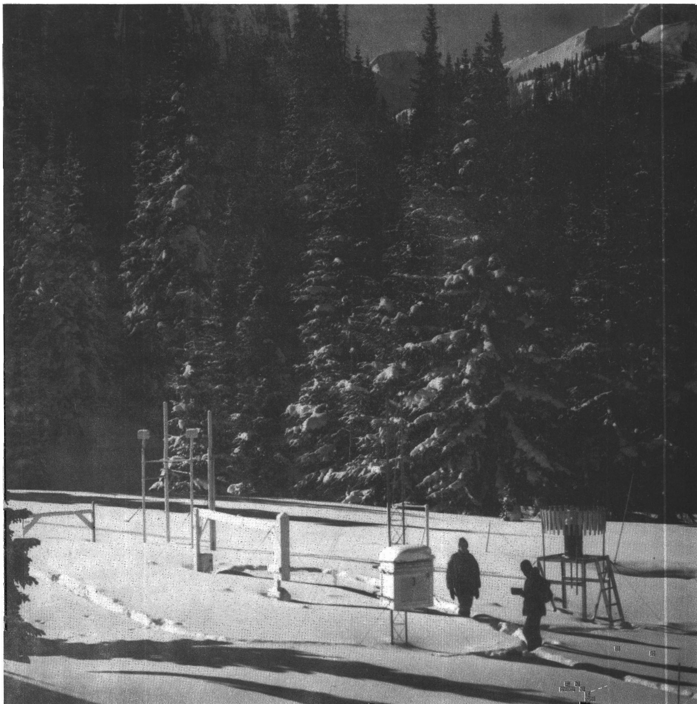
Figure 8. Part of the snow study plot at Red Mountain Pass. From right to left instrumentation includes: recording precipitation gauge with Alter shield; standard meteorological screen; "zig-zag" isotopic snow profiler (immediately behind screen); snow settlement gauge; isotopic snow profiler (4 upright posts and connecting limbs); fixed thermocouple array. The three snow boards, master stake and data read-out shack are off the picture to right.
