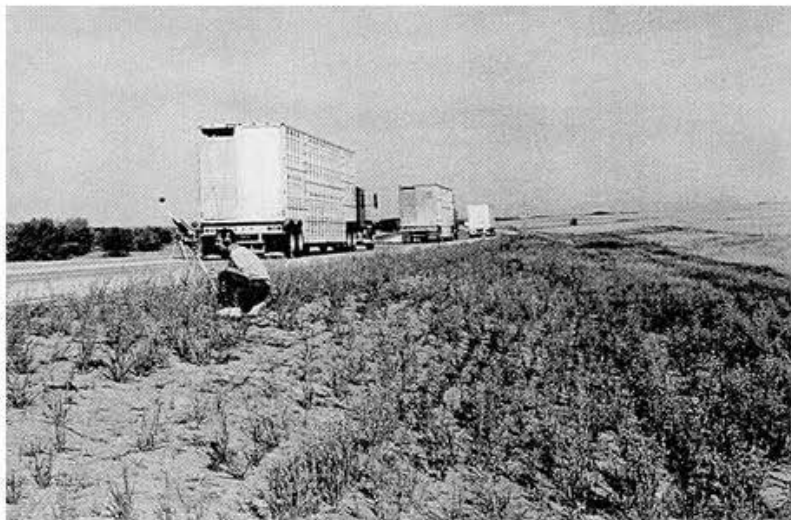
Photo 26: Acquiring truck noise levels at the roadside
