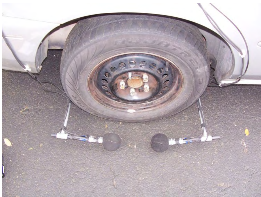
Figure A.2. OBSI Measurement Bracket Configuration.
