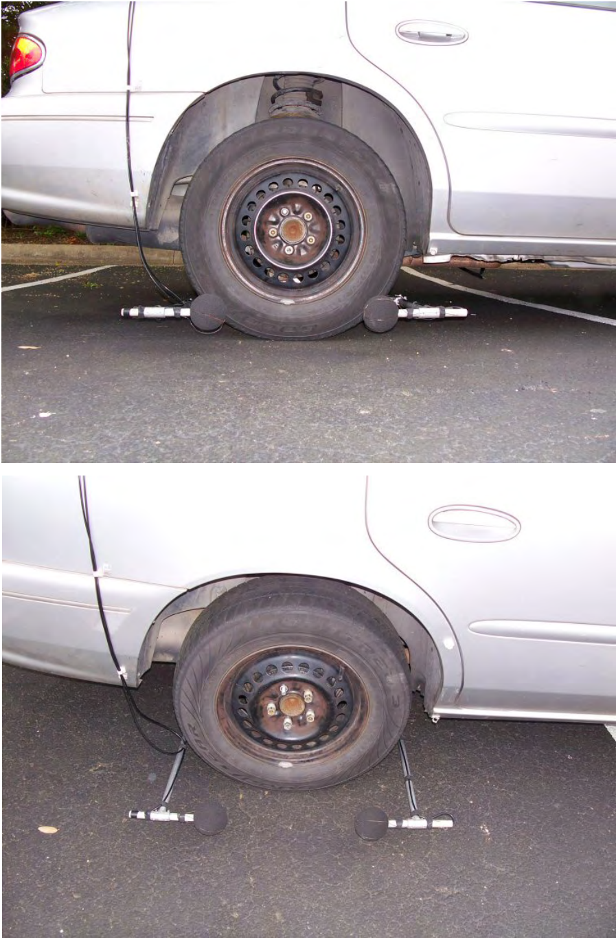
Figure A.1. CPX Measurement Bracket Configuration.
