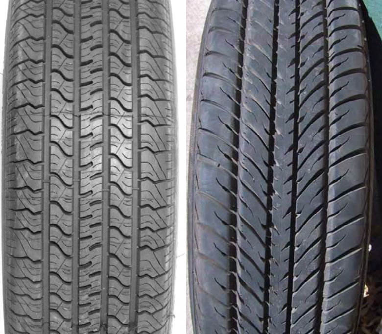
Figure A.3. Test Tires – ASTM F 2493 SRTT and Goodyear Aquatred III.
