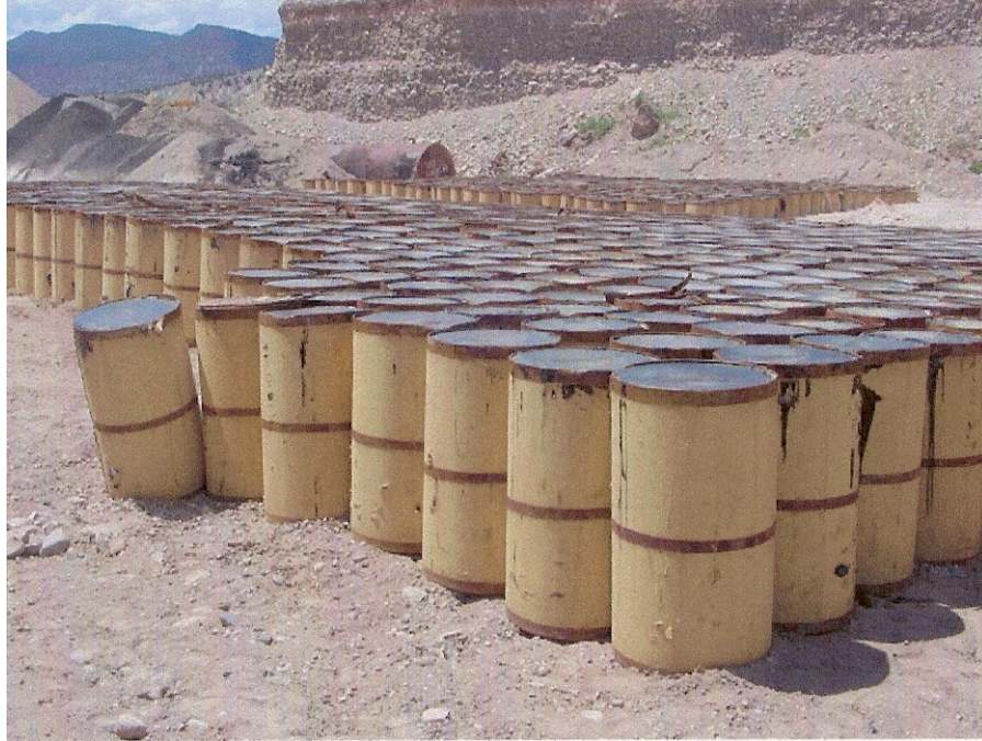
Figure 6. Trinidad Lake Asphalt Delivered to Project
