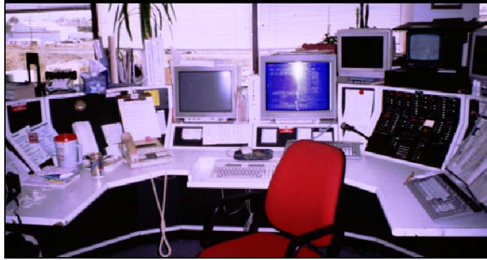
Figure A-4 CAD, AVL and Legacy VAX Equipment at a Dispatcher's Console
