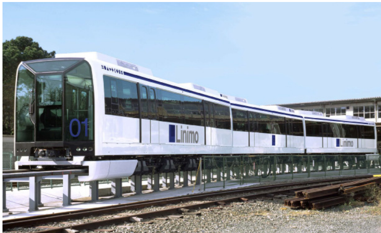
Figure A-1: CHSST Linimo Maglev Vehicles (Low Speed) for the Tobu Kyuryo Line in Nagoya, Japan
