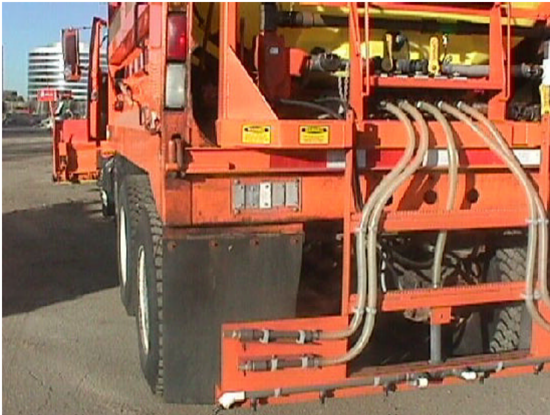
This CDOT Maintenance chemical deicing distributor truck has five test “coupons” (steel squares) mounted on the back of the truck to determine corrosion rates due to chemical deicing.
