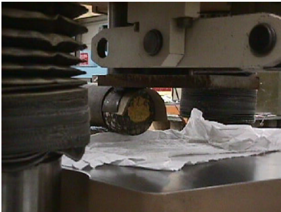
The pavement sample being tested was soaked in magnesium chloride before an overlay was added. This machine is testing the sample for shear strength.
