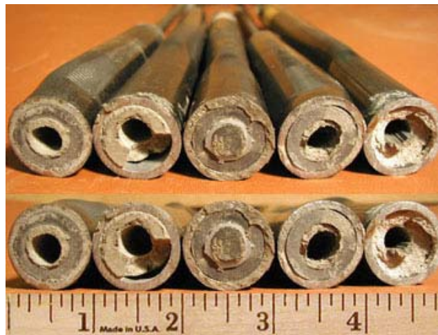
Figure 3.4 - Unconditioned CFRP Grip Failure
