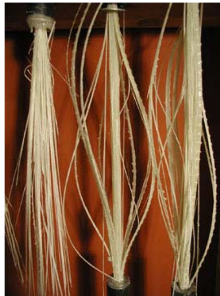
Figure 3.6 - Failure Mode of 3/8" GFRP S
