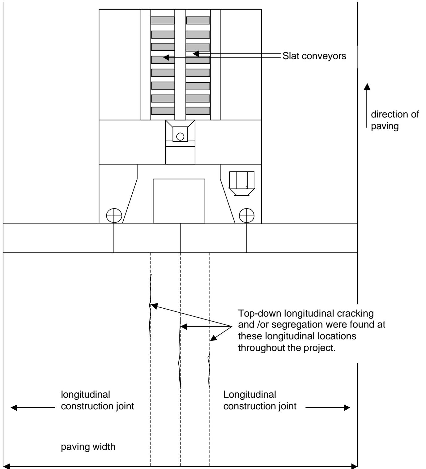
**Table D. Paver manufacturer/model and location of longitudinal cracking**
