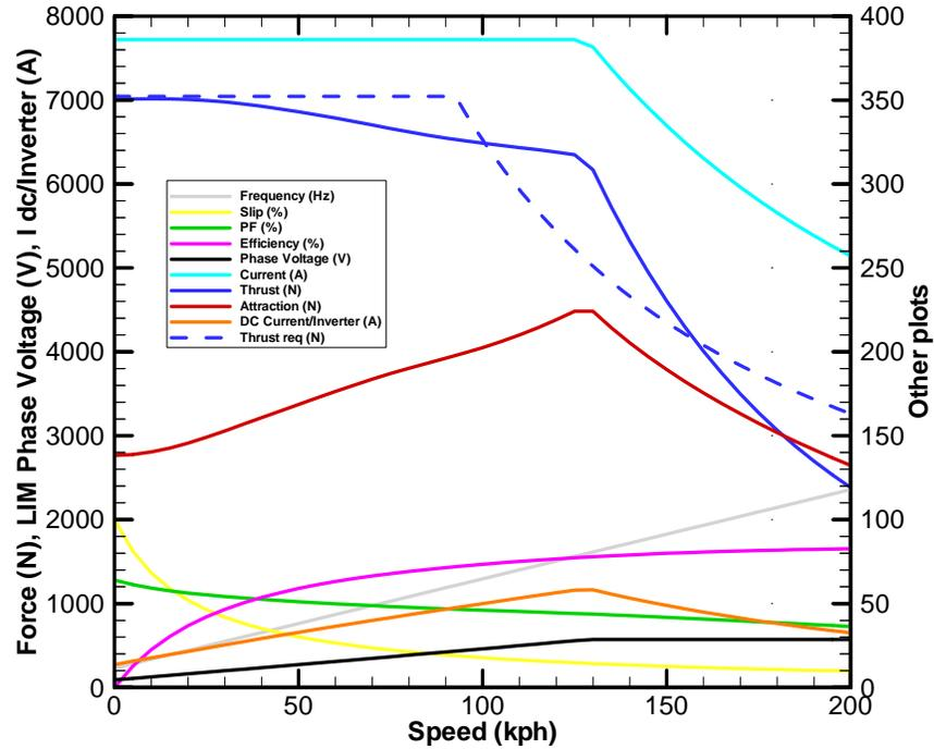
**Figure 75: Performance curves for COL-200 LIM with updated spatial harmonics analysis code using parameters labeled 19nov03a in Table 6-2. DC current per inverter is for one inverter feeding the 5 LIMs in a 1 series – 5 parallel configuration. Two inverters are in series per car hence drawing the same trolley current per car.**
