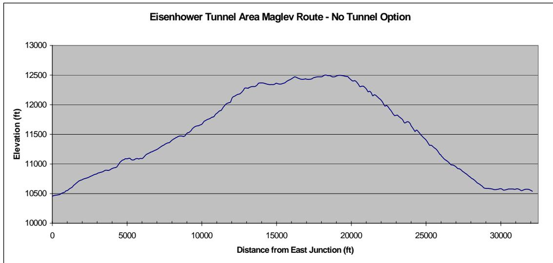
**Figure 34: EJMT Alternative (No Tunnel) Elevation Profile**
