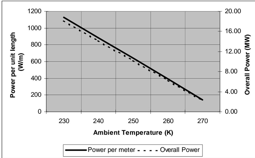
**Figure A.5.11: Heater power per meter required to maintain the third rail above 274 K as a function of ambient temperature. Overall heater power refers to the 3rd rail heater power required for a 16 km (10 mile) section of track, two rails, one source and one return.**
