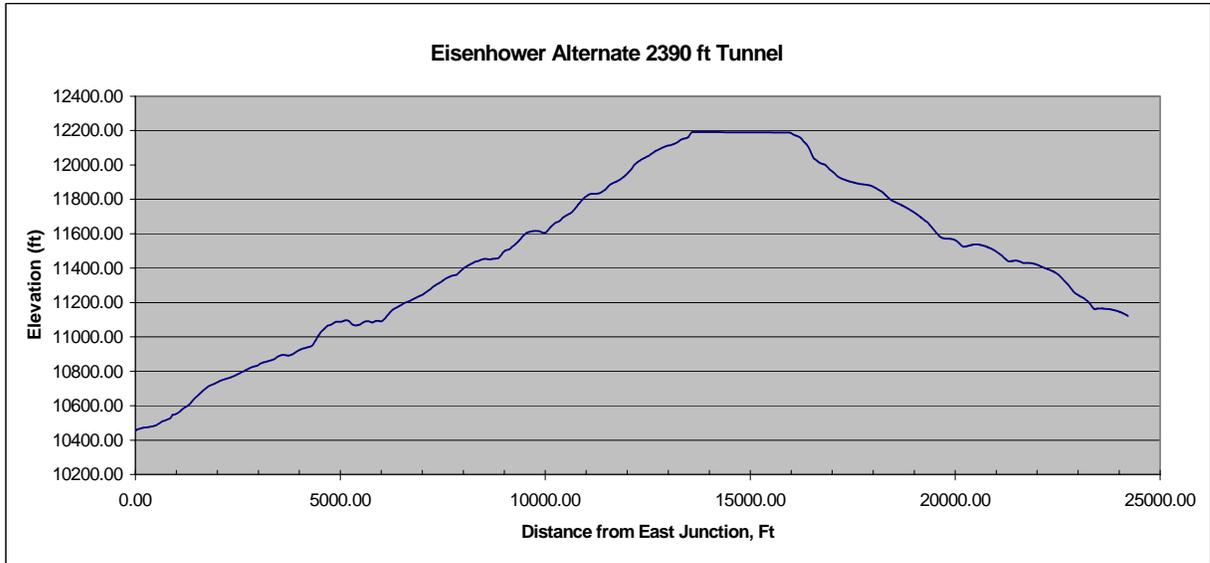
**Figure 31: Eisenhower Alternative 2390 foot Tunnel Elevation Profile**
