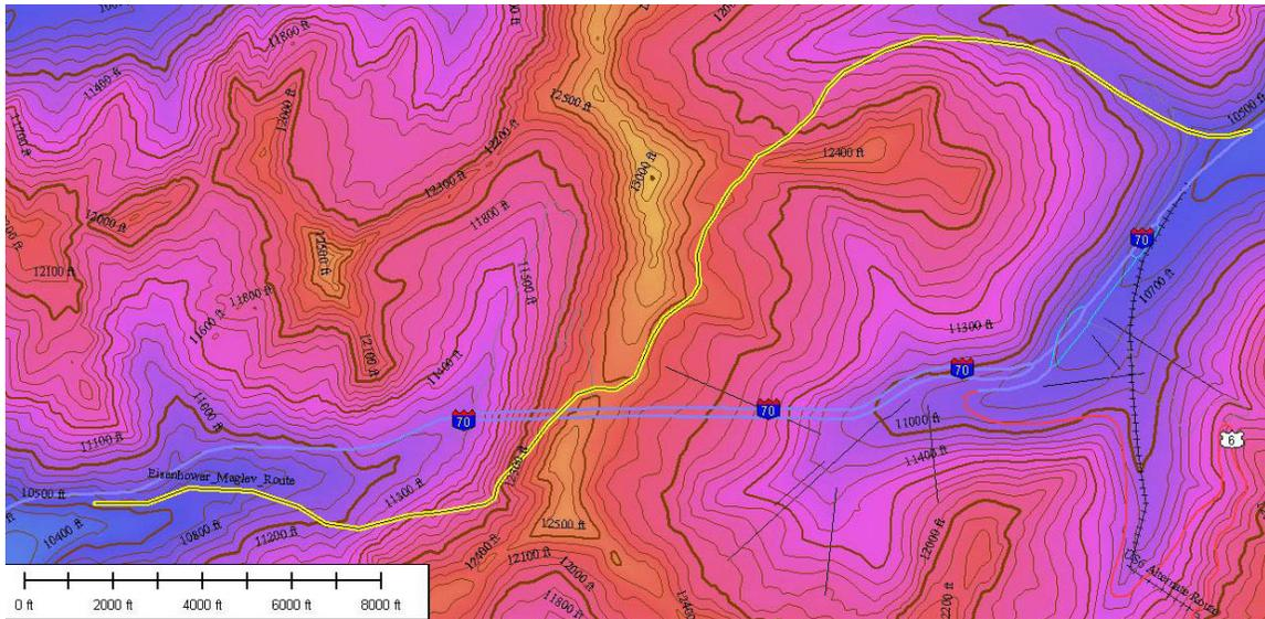
**Figure 33: EJMT Alternative Maglev Alignment with No Tunnel**
