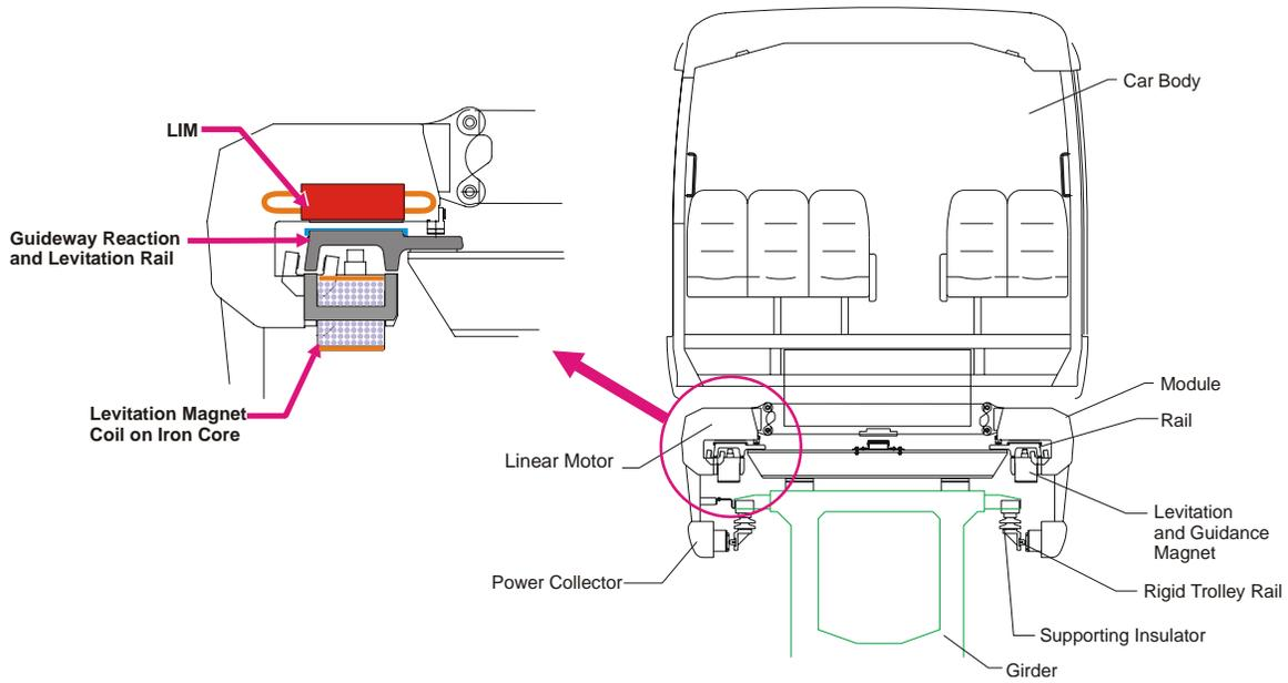
Figure 86: Close-up of propulsion/levitation module for LIM.
