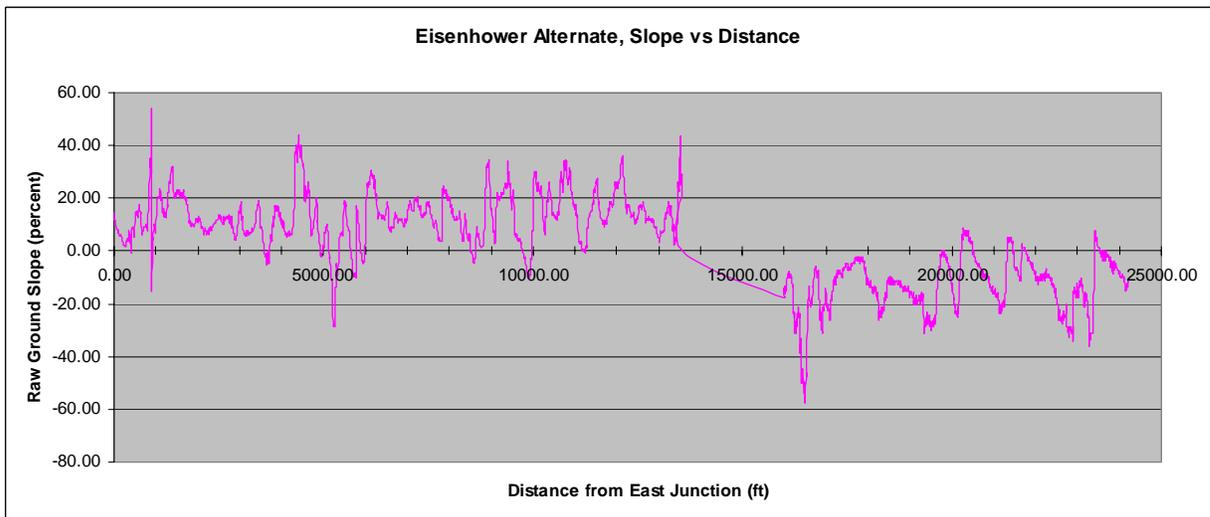
**Figure 32: Eisenhower Alternative 2390 foot Tunnel Slope Profile**
