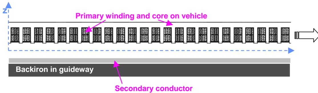
Figure 87: Side-view, cross-section of single-sided LIM components.
