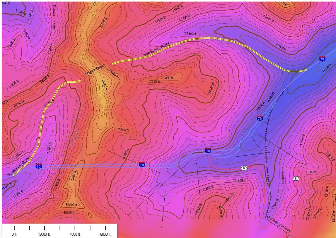
**Figure 30: EJMT Alternative Alignment, with Short Tunnel**
