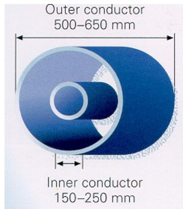
**Figure 54: Cross Section of Siemens GIL**
