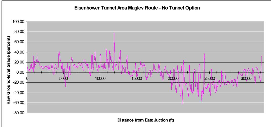
**Figure 35: EJMT Alternative (No Tunnel) Slope Profile**
