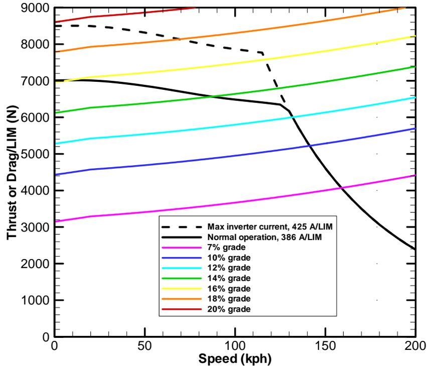
**Figure 77: Thrust per LIM at normal operating current of 386 A and maximum inverter output. Drag force/LIM curves for married pair of COL-200 vehicles on various grades into a 90 kph headwind at zero acceleration.**
