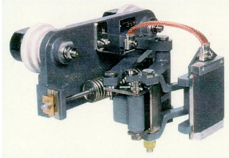
**Figure 82: Spring contact pantograph of power collector**
