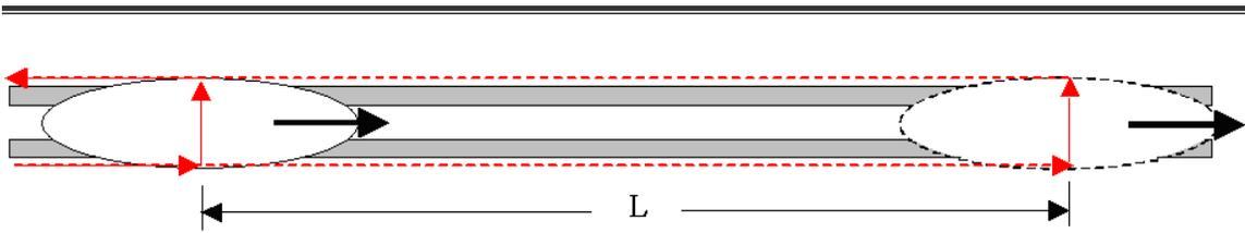
**Figure A.5.8: Schematic of current flow from the substation to the vehicle as it moves down the track.**
