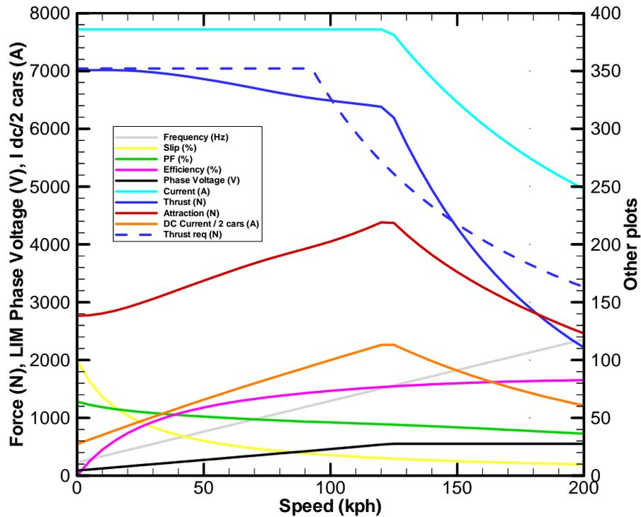
**Figure 74: Performance curves for COL-200 LIM with updated spatial harmonics analysis code using parameters labeled 11oct03b in Table 6-2. DC current per 2 vehicles is for all inverters feed the 20 LIMs in a 4 series – 5 parallel configuration.**
