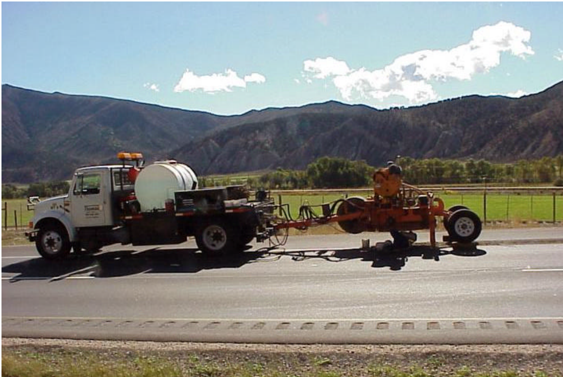
Figure 3. The equipment used to grind the standard rumble strips. The operation is stopped and the trailer raised so the operator can replace worn teeth on the grinding drum.
