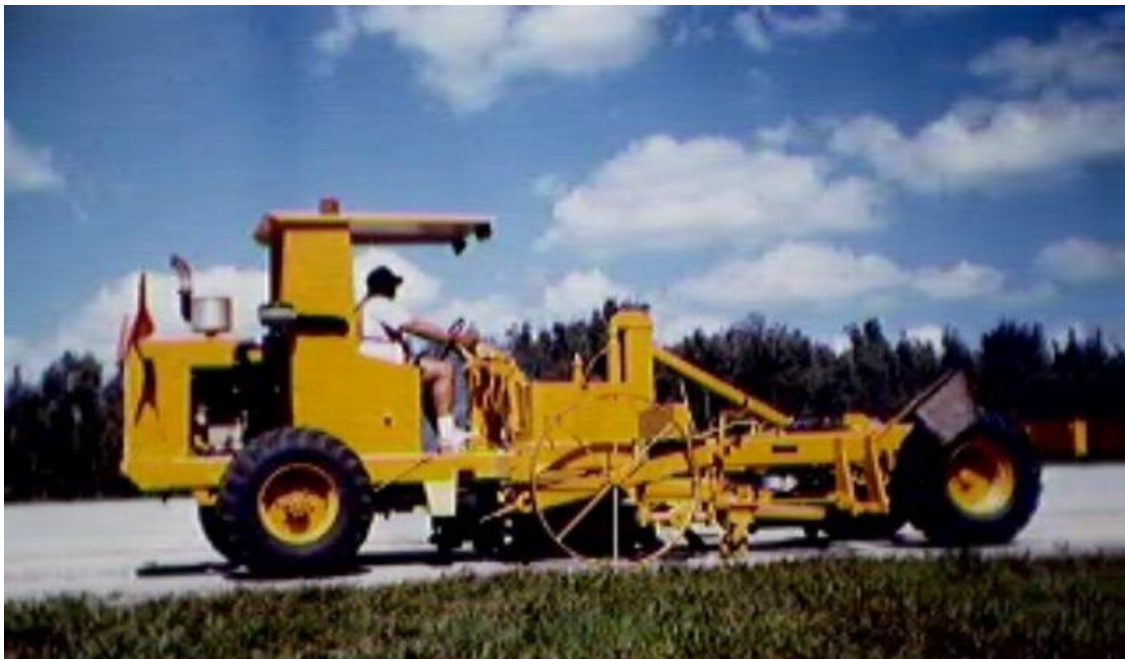
Figure 10. The machine used to make the two-inch-groove rumble strips. The grinding drum is located near the center of the machine and moves from the operators left to his right to grind the grooves. The drum is six feet long so the machine grinds six feet of rumble strip at each stop.
