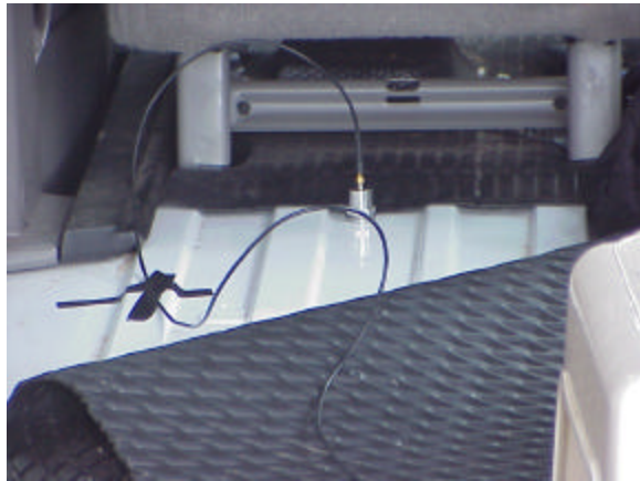
Figure 26. An accelerometer was mounted to the floor of the van.
