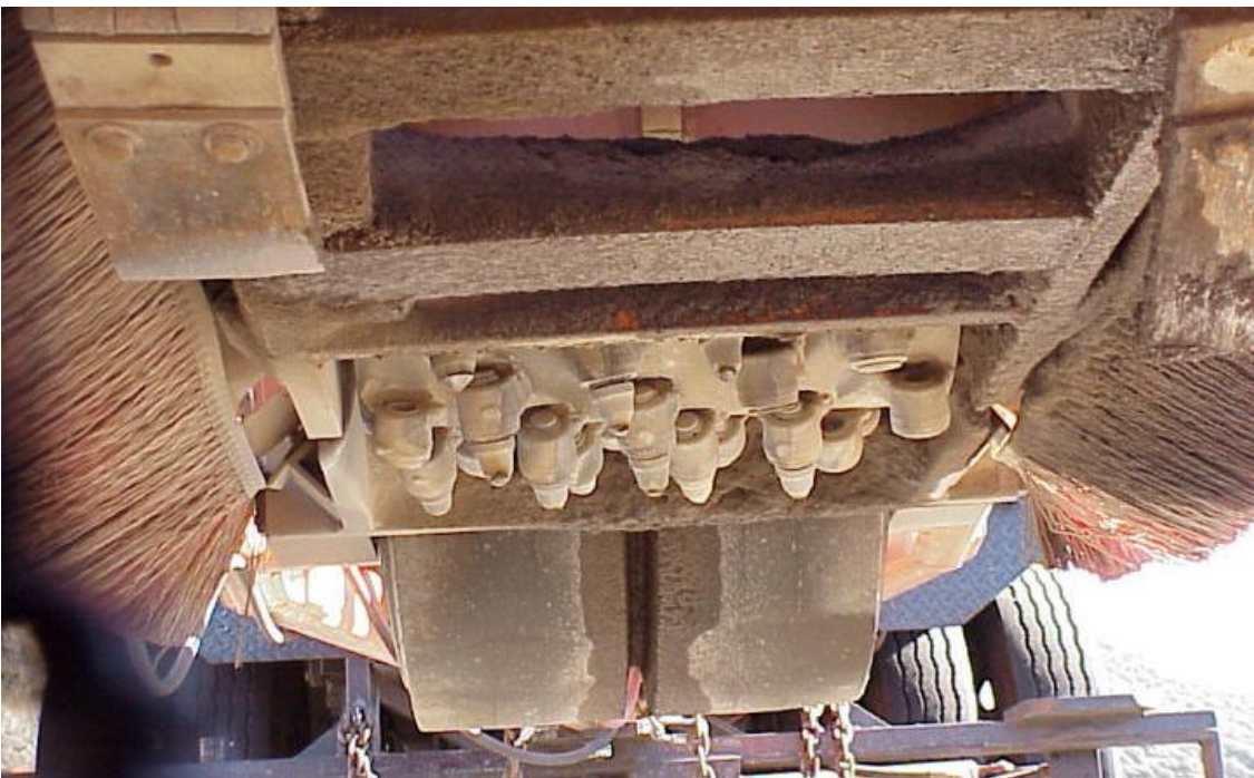
Figure 6. The underside of the grinder trailer. This shows the grinding drum with its teeth. Notice the empty sockets at the right of the drum. By adding more teeth or taking some out the length of the grooves - the width of the rumble strip can be adjusted. The lateral offset in the teeth causes the rough texture of the grooves.
