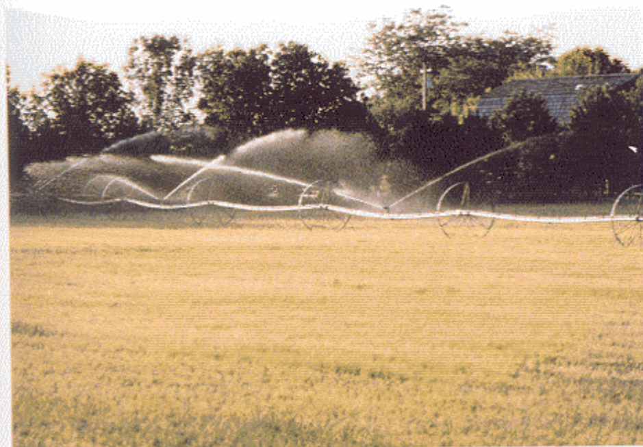
Side-roll irrigation system for hay production Photo by William Cotton, Colorado State University
