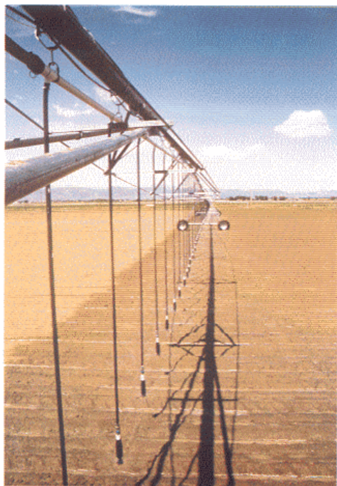
Low pressure drop nozzels reduce drift loss and increase application precision. Photo by Grant Cardon, Colorado State University
