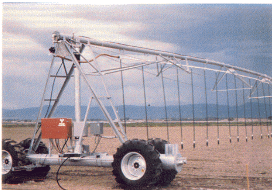
Linear move sprinkler system. Photo by Grant Cardon, Colorado State University
